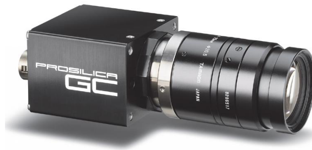
Figure 21 Prosilica GC1380C camera (Allied Vision Technologies, 2013)
