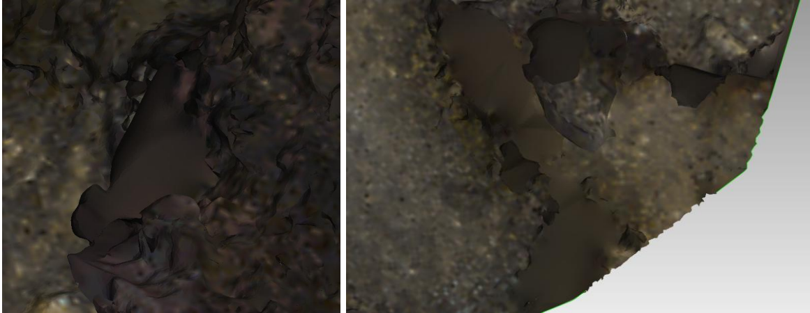
Figure 56 Holes filled by the tangent (1) and the flat (2) technique
