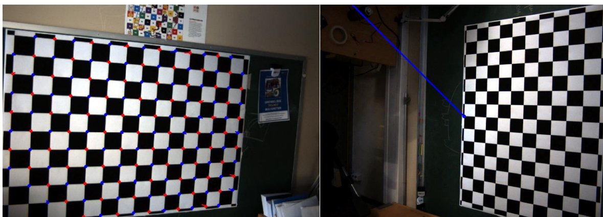
Figure 35 The horizontal and the rotated image with the measured image points in the AgiSoft Lens.
