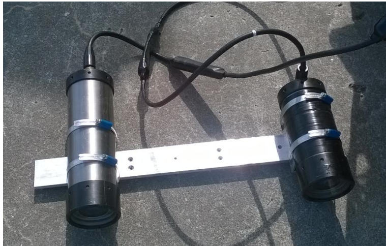
Figure 25 The camera housings n the new stereo bar
