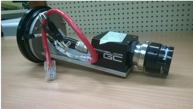
Figure 23 Inside of the second camera housing with connection cables
