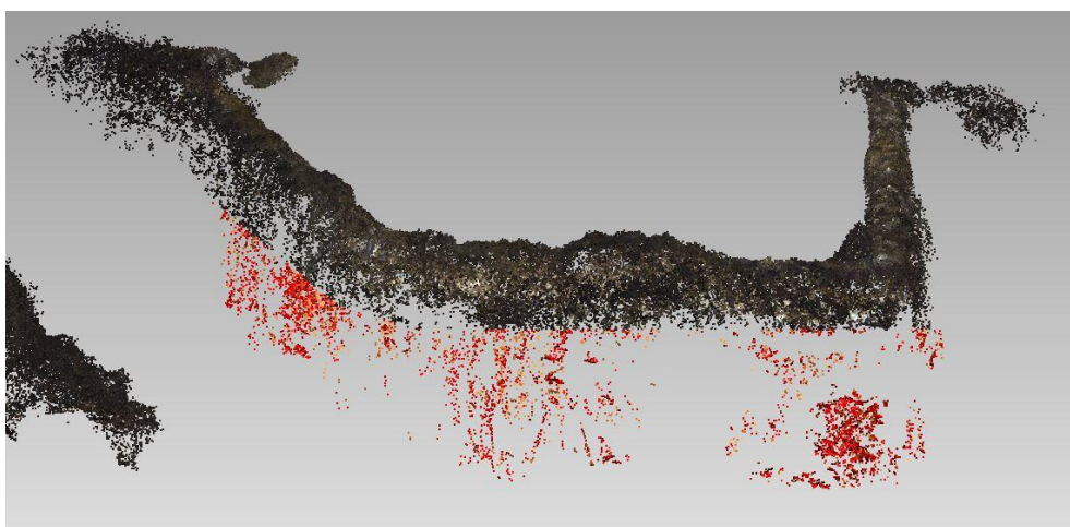
Figure 53 Removal of the seaweed from the underwater model
