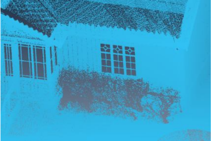
Figure 3.41. Point cloud without bushes in front of the house-PolyWorks.
