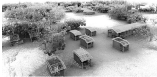
Figure 2.10. a: Point cloud of the Peel Island Lazaret generated from ' Zebedee ' data, b: aerial view of rendered Zebedee point cloud, the point cloud has been subsampled to 9% of the original data. (Source: [25])
