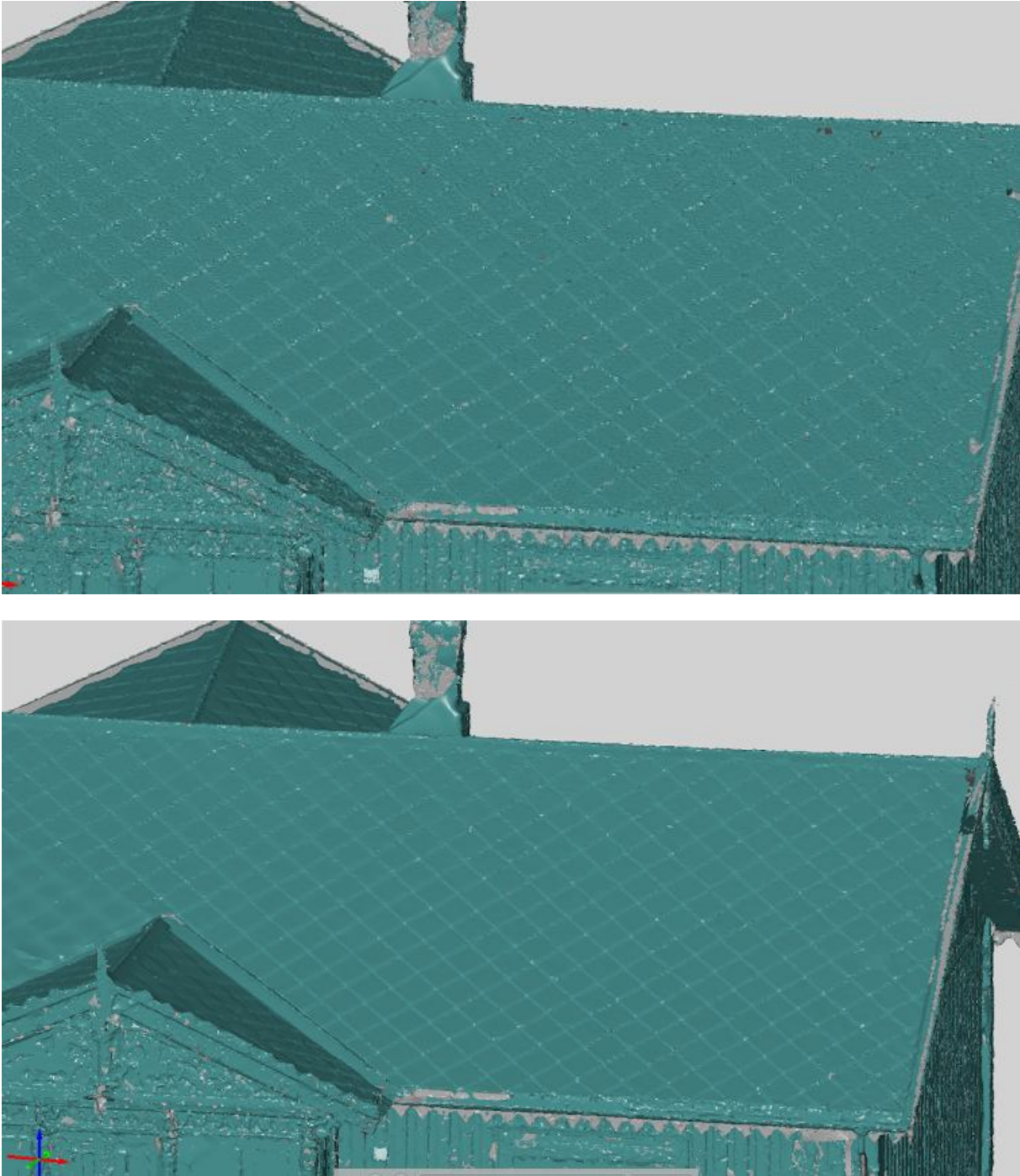
Figure 3.81. Part of the house before (up) smoothing and after (down) the operation. GOM Inspect.
