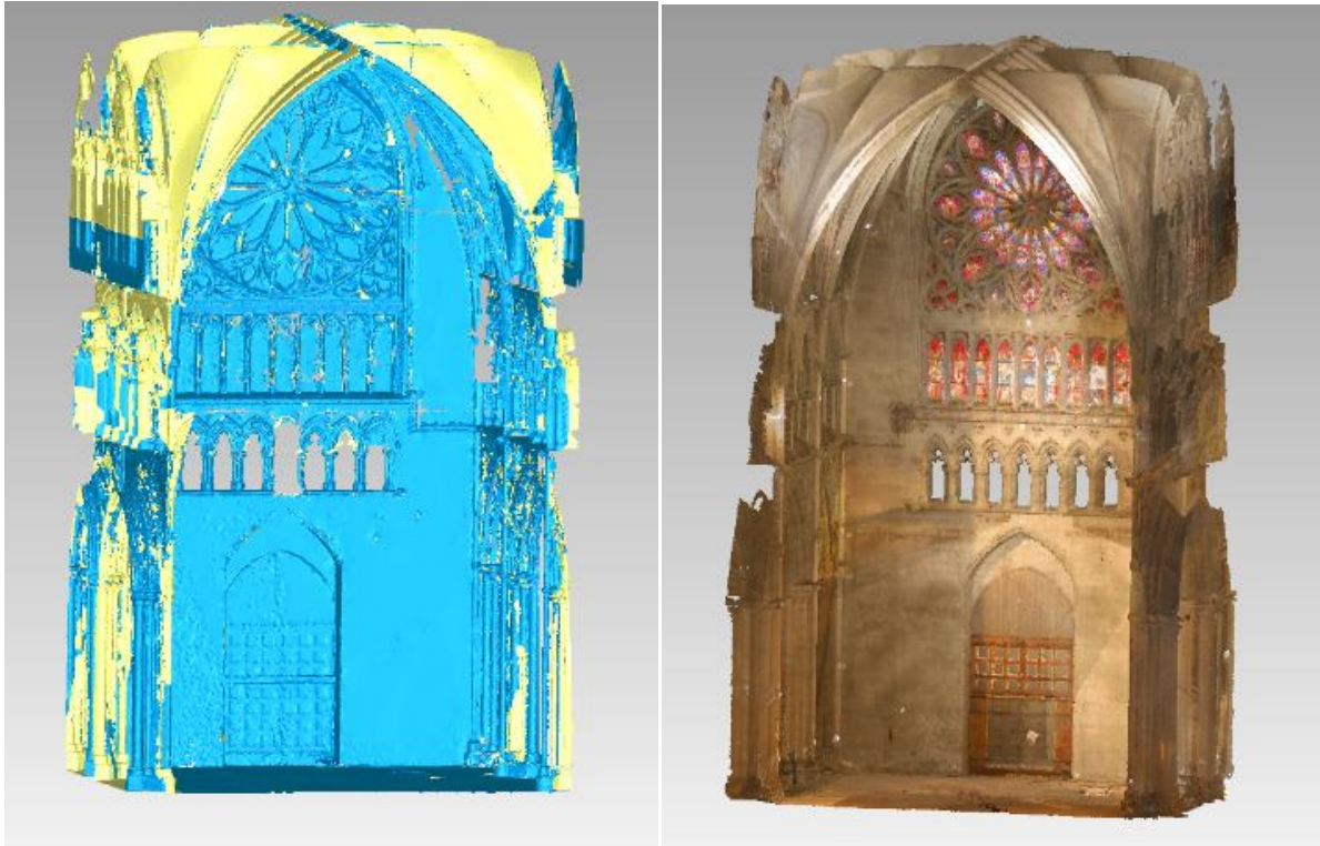
Figure 3.63. Left :model created in PolyWorks, right: point cloud from RiScan PRO.
