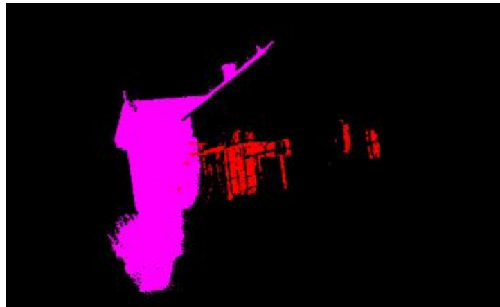
Figure 3.21. Manual cleaning of window's reflections.
