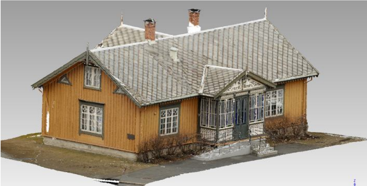
Figure 3.87. Textured front of the house with bushes projected onto walls, displayed in Geomagic.
