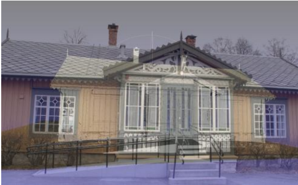
Figure 3.89. Raster registration within the MeshLab software.
