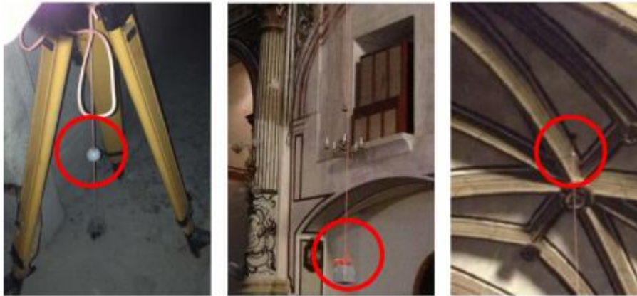
Figure 2.12. Plumb line system used to reference all three models together, left: tripod with a plumb line inside of the vault, middle: plumb line from inside of the church with the load, right: plumb line from inside of the church with spheres (Source: [6])
