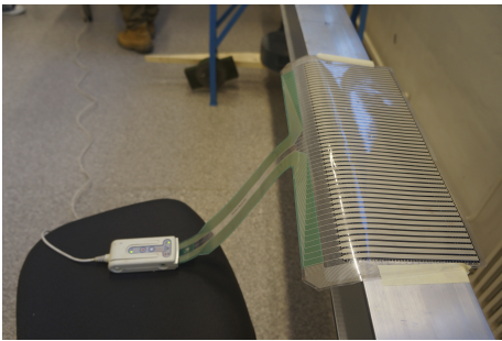
(a) Sensor were connected to the aluminum section using tape.
