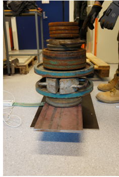
(a) Steel wights used to load the sensor during calibration.
