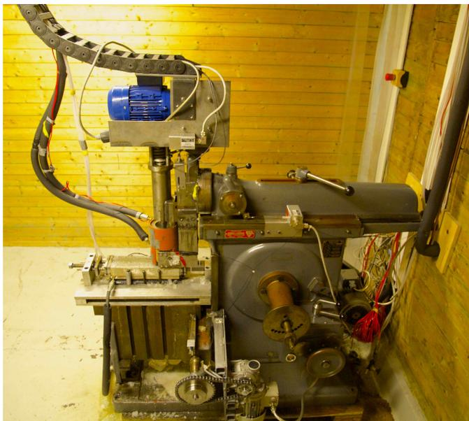
Figure 3.11: Ice-concrete abrasion rig.
