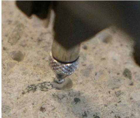
Figure 5.4: Mitutoyo indicator needle hanging on a cavity wall. The needle tip measures 1.8 mm in diameter.
