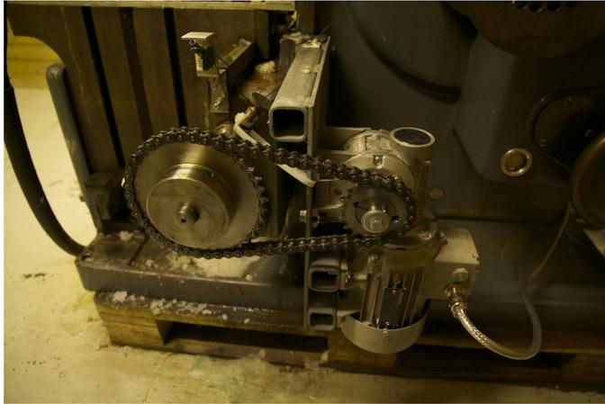
Figure 3.14: Automatically adjustment of table with new motor
