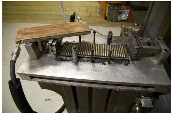
(b) Copper "sandwich" to the left and roll bearings are seen to the right of it. Horizontal load-cell further to the right.
