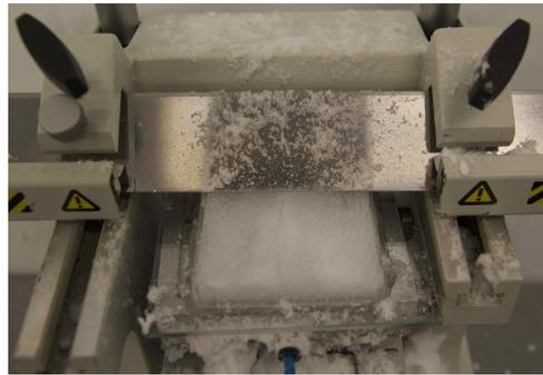
(d) Collapsed center of sample c13's vertical section, (Procedure 4)
