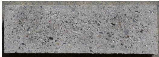
(d) Concrete sample D7 exposed to ice made after procedure 4.
