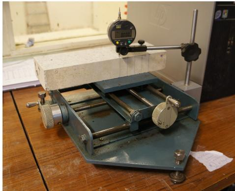
Figure 3.15: Abrasion depth measurement set-up for initial reference point. From bottom to top: Coordinate table, concrete specimen and digital indicator. Rotation wheels are seen in front and on the left side of the coordinate table.
