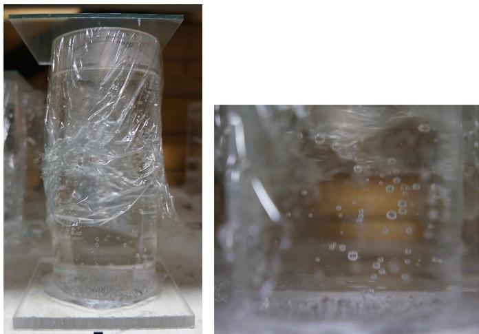
(a) Prepared sample. Glass plate seen on top of the sample, plastic foil wrapped around top part of sample. (b) Close up of figure 3.4a. For scale: Edges of tube seen on either side of the figure. Gas bubbles inside the tube are clearly seen.
