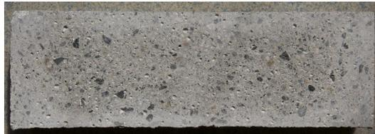
(e) Concrete sample D6 exposed to ice made after procedure 5.
