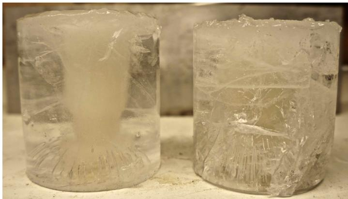
Figure 5.6: Comparison of intact p2 POM,  $\phi = 73.5$  mm, sample (left) and broken p1,  $\phi = 70$  mm, ice sample (right) after an ice-concrete abrasion test. Abraded surface on top.
