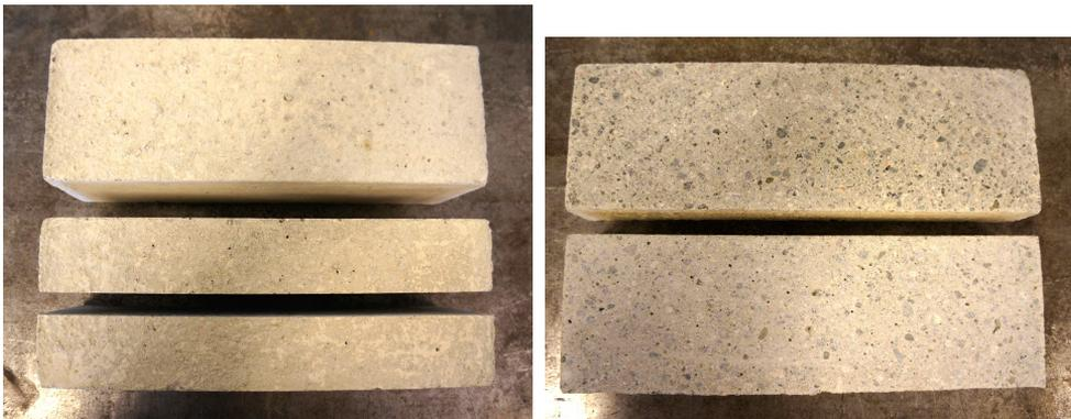
(a) Top: Before sawing. Bottom: After sawing. (b) Top: Before honing. Bottom: After honing.
