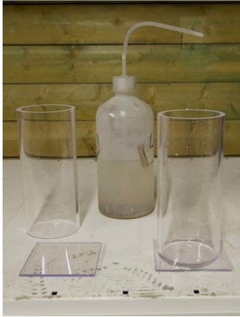
(a) Plexiglas parts. Water squirter used to pour water along the edge in the middle. Figure from Greaker (2013).
