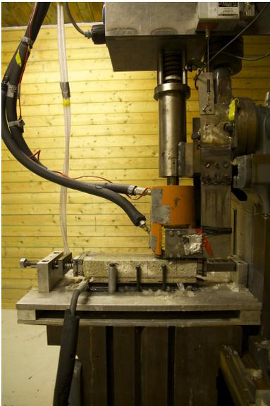
(a) Piston. Vertical piston attached to the motor and container. Concrete sample on copper "sandwich" underneath container.
