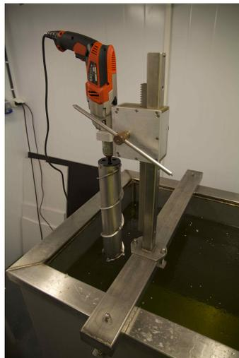
(b) Assembled rack, drill and core
