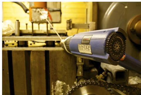
Figure 5.7: De-icing of load-cells. Industrial dry blower blowing air at a temperature of  $\approx 150$  °C at the load-cells seen under the table holding the bearings. Load-cell A to the right and load-cell B to the left.
