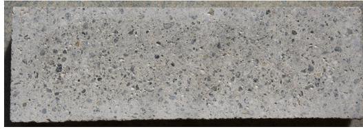
(a) Concrete sample STD9 exposed to ice made after procedure 1.
