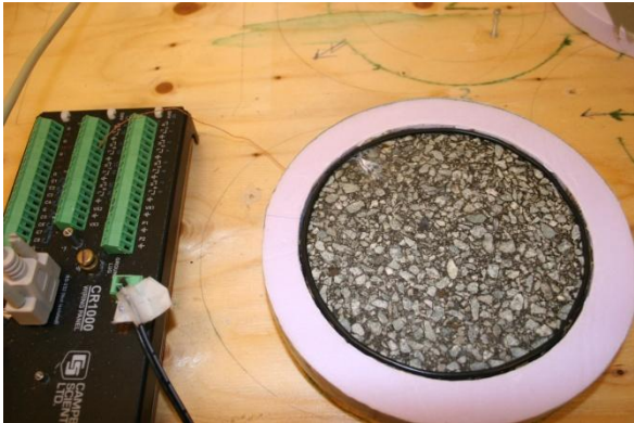
Figure 6 – Substrate connected to the data logger
