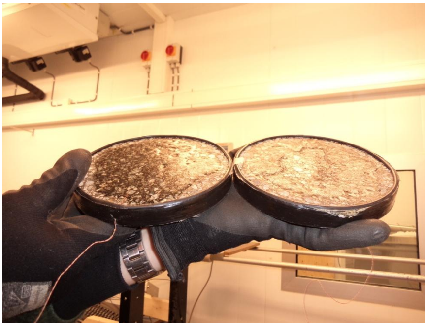
Figure 10 - Substrates after testing with British Pendulum Tester
