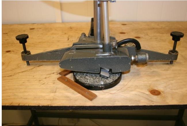
Figure 9 - Setup for testing of a solution with the British Pendulum Tester
