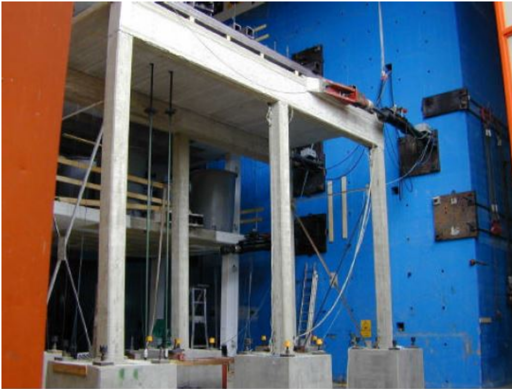
Figure 4.2: One-story reinforced concrete building (Ferrara & Negro, 2003).
