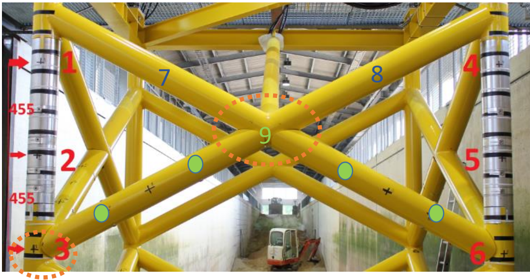
Figure 5.8: Front view of the front instrumented bracings and instrumented columns.
