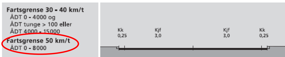
Figure 42: Second condition of Road with two lanes driving (Statens Vegvesen, 2008)
