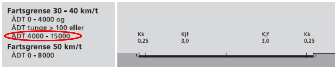
Figure 41: Second condition of Road with two lanes driving (Statens Vegvesen, 2008)
