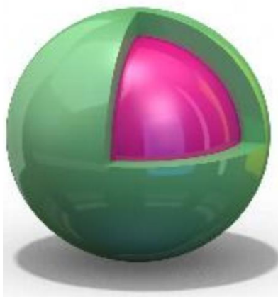
Figure 3 Model of a microencapsulated PCM with a wax core and polymeric shell (Phase energy [81]).
