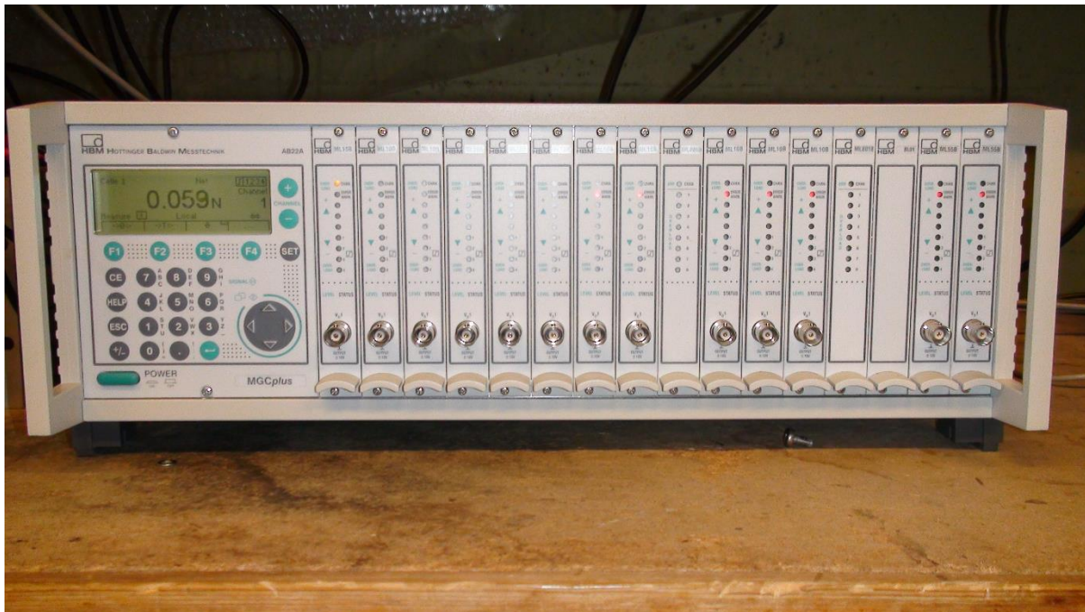
Figure 3.10: HBM MGCplus amplifier system
