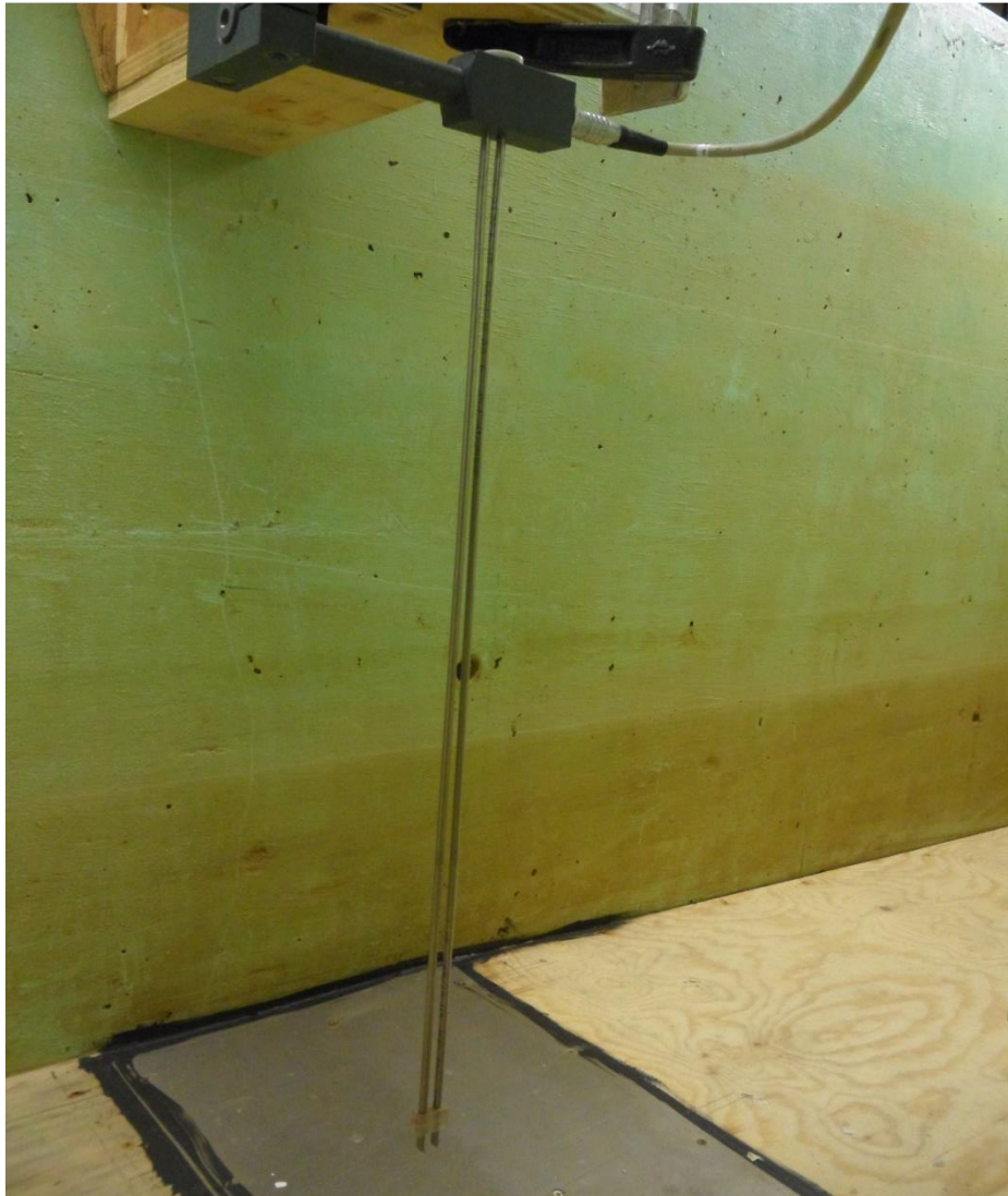
Figure 3.4: A picture of a wave gauge used in the experiment
