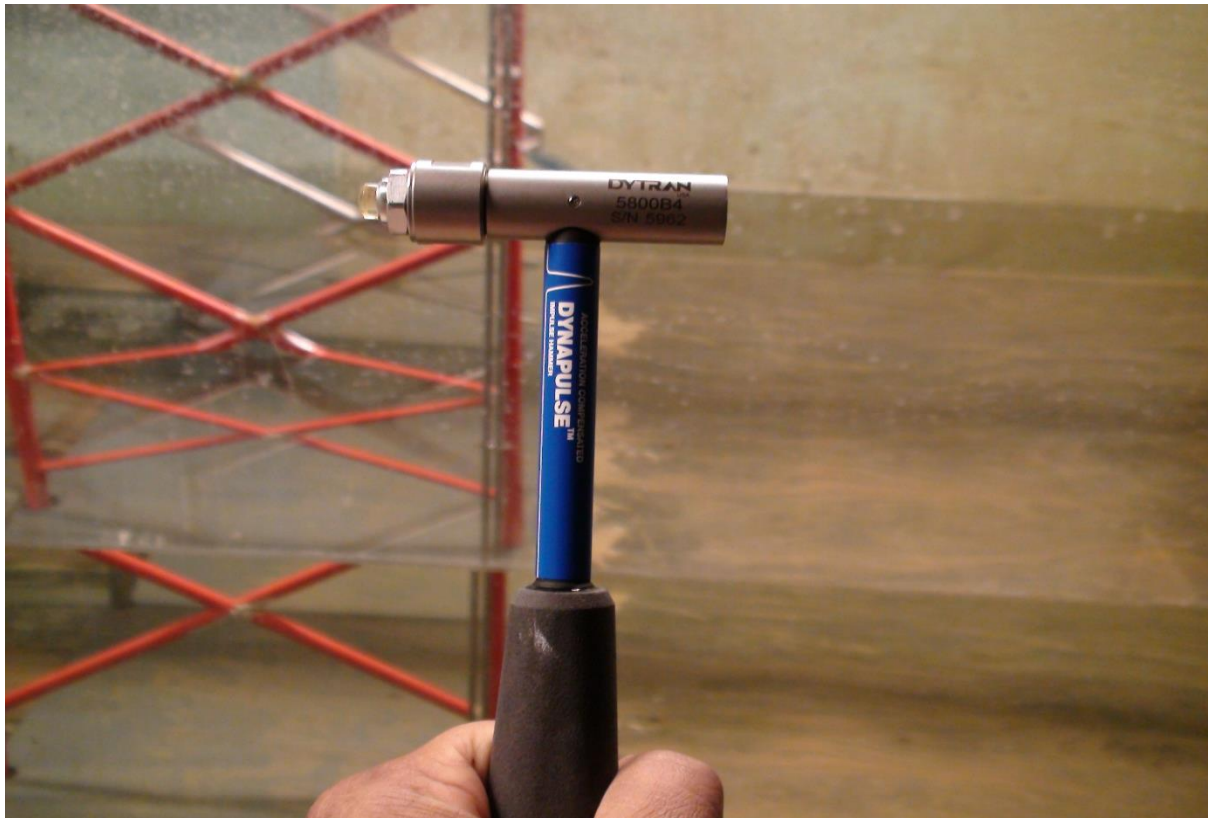
Figure 3.6: A picture of an impulse hammer used in the experiments
