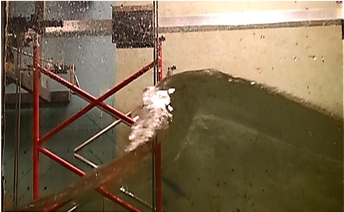
Figure 4.23: Snapshot from test 'Ue480t196' on side section of the truss structure
