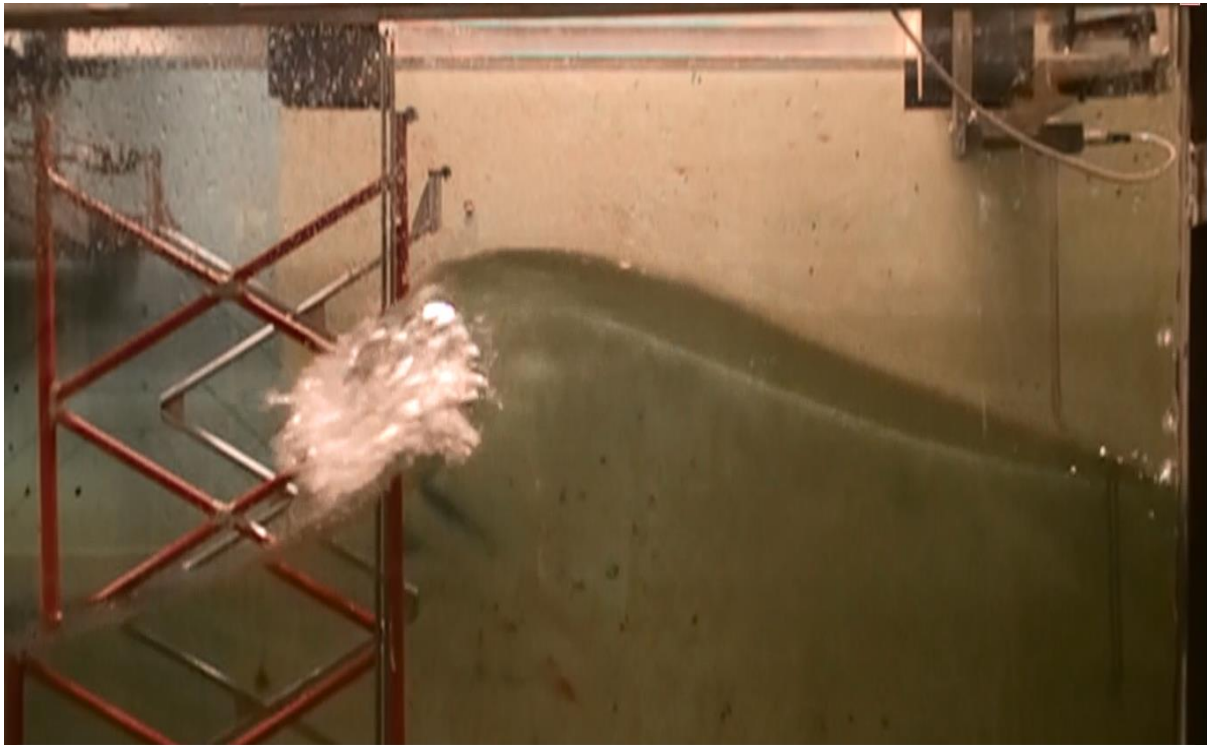
Figure 4.27: Snapshot from test 'Ue500t208' on side section of the truss structure
