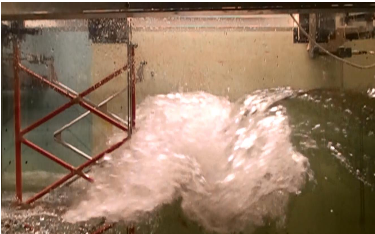
Figure 5.6: Snapshot from test 'Ue610t196' on side section of the truss structure
