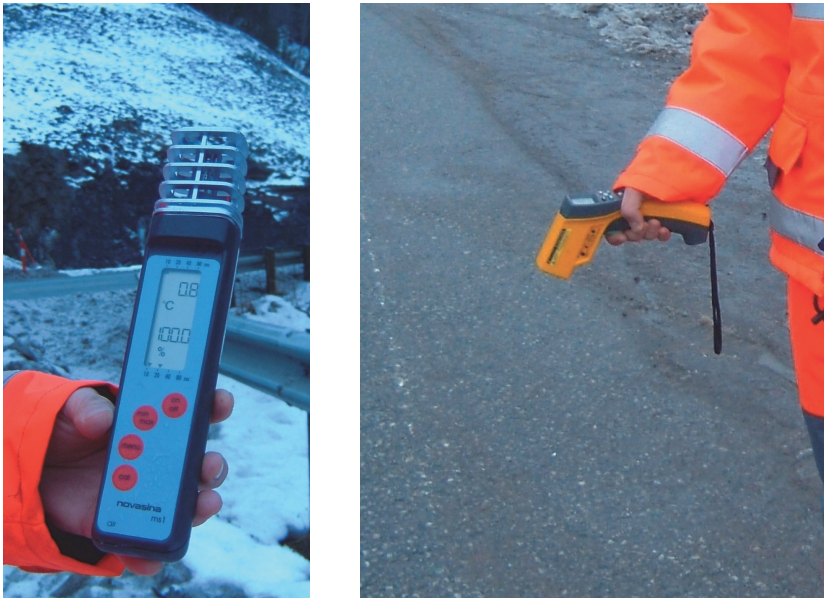
Figure 5.8 Measuring air temperature and humidity and road surface temperature.
