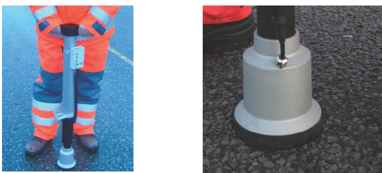
FIGURE 2 Measuring quantity of salt on road surfaces with the Sobo 20.
