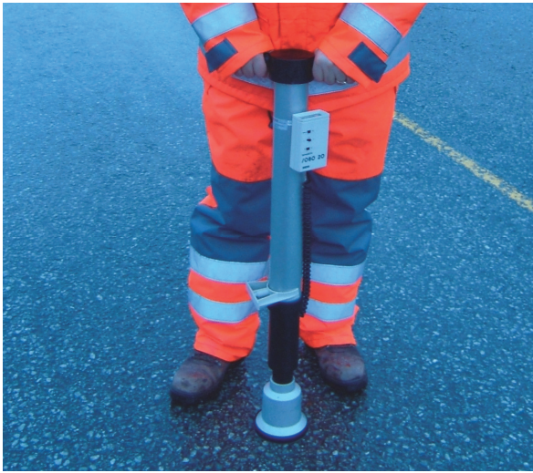
Figure 6.2 The use of the Sobo 20 on a road surface.
