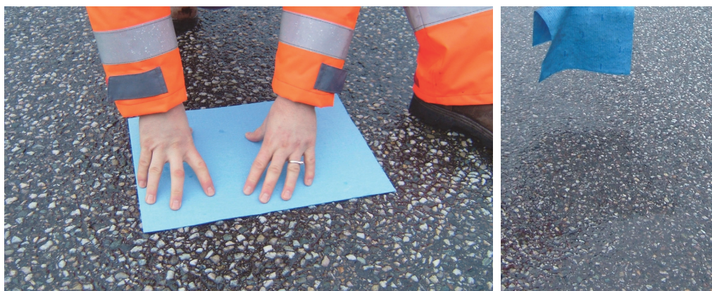
Figure 5.7 Measuring quantity of water on road surfaces with Wettex.
