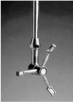
Figure 31 Side looking 3D probe
