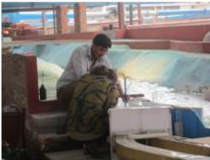
Figure 36 MicroPropeller measurements at the intake of the PHM of LMM HPP
