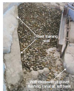
Figure 76 River training structures Khudi model (Shrestha et al., 2008)
