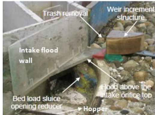
Figure 73 Modifications at the intake of PHM of Khudi HPP (Shrestha et al., 2008)
