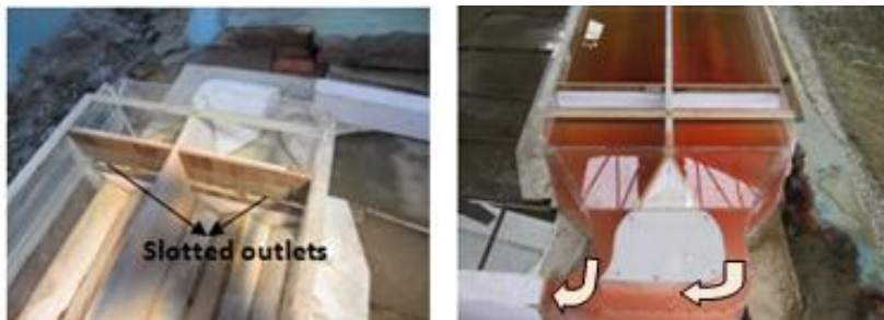
Figure 28 Final arrangement on the Settling Basin outlet in the PHM of LMM HPP
