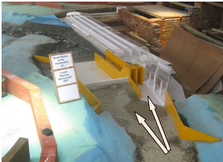
Figure 18 Initial physical model of the headworks of LMM HPP (Shrestha and Bogati, 2012)
