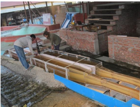
Figure 32 ADV measurements along the settling basins of the PHM of LMM HPP
