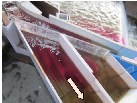
Figure 19 Final arrangement of the intake of the PHM of LMM HEP
