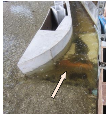
Figure 23 Bed Control at the final arrangement of LMM HPP
