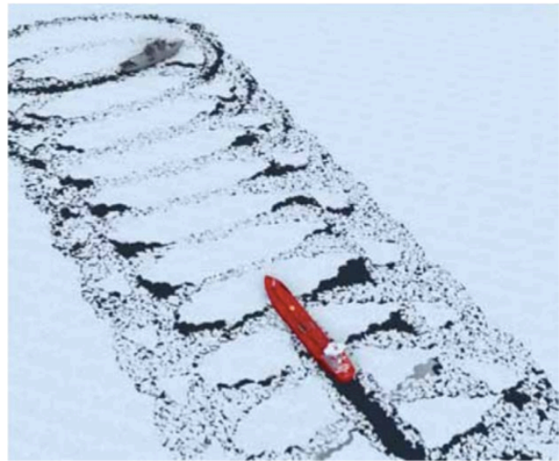
Figure 1-3 Ice breaker assisted tanker on dynamic positioning (Metrikin et al., 2012b/ www.smsc.no )
