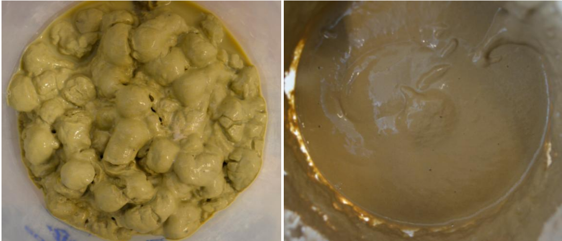
FIGURE 6.9: HYDRATED BENTONITE PELLETS AFTER 72 HOURS (LEFT). THE RESULT OF MIXING DESCRIBED IN POINT 2 AND POINT 1 (RIGHT)
