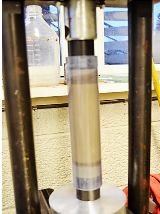
FIGURE 7.8: THE MUD INSIDE PIPE IN A MECHANICAL COMPRESSOR. NOTICE THE WATER DRAINING FROM BENTONITE MUD AND INTO SAND FILTER AT BOTH ENDS OF THE PIPE.
