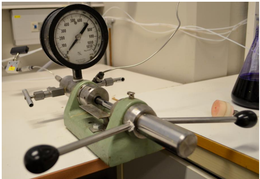
FIGURE 6.2: RUSKA PUMP USED TO INJECT COLORED WATER INTO PIPE FILLED WITH BENTONITE AND SAND
