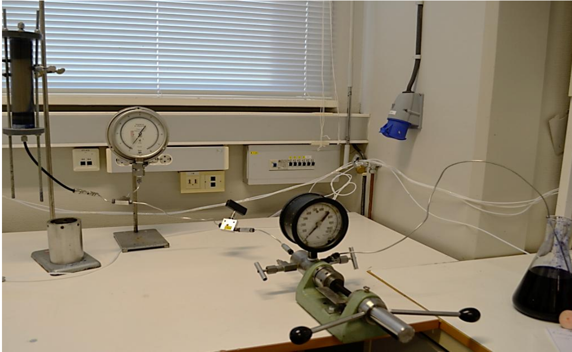
FIGURE 6.11: THE MAIN EXPERIMENTAL SETUP. COLORED WATER, BLUE, IS FEED TO THE PUMP, WHICH INJECTS IT INTO THE PIPE FAR TO THE LEFT WHILE CONTINUOUSLY MONITORING THE PRESSURE IN THE MUD COLUMN WITH A PRESSURE METER (LEFT TO THE CENTER IN THE PICTURE)
