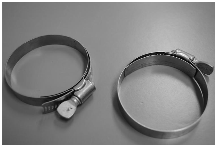
FIGURE 7.6: HOSE CLAMPS USED TO RESTRAIN THE PVC PIPE EXPANSION
