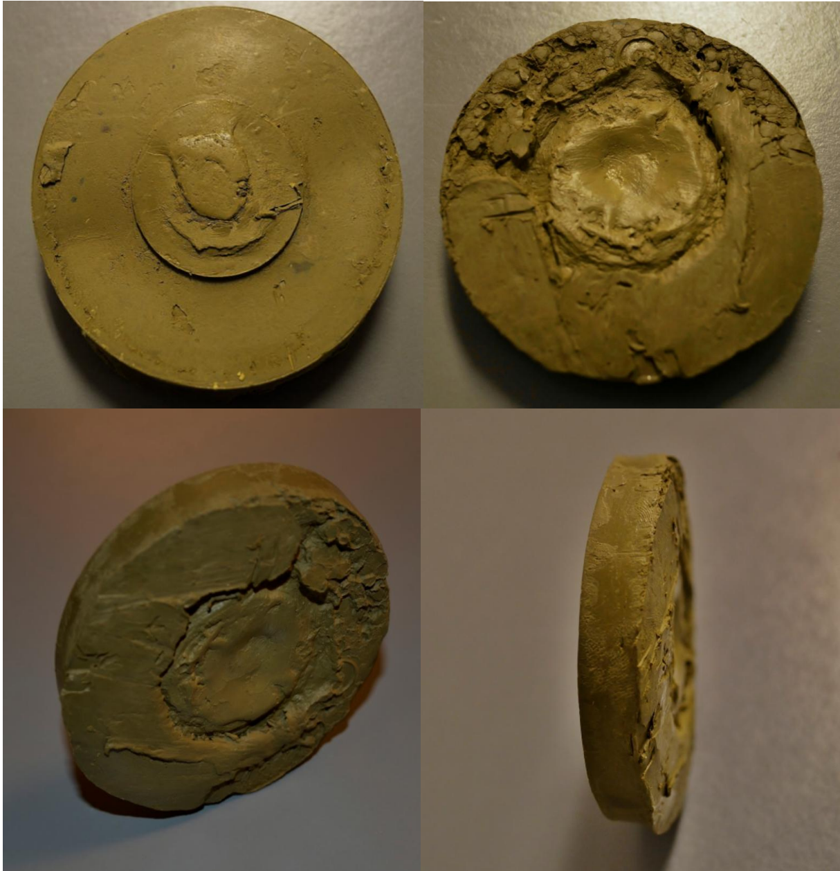
FIGURE 7.14: THE SAMPLE, AT THE END OF TESTING. THE UPPER LEFT PICTURE SHOWS THE SAMPLE AS IT WAS IN THE HOLDER, THE DAMAGES SEEN ON THE PICTURE UPPER RIGHT COMES SOLELY FROM THE OPERATION OF GETTING THE SAMPLE OUT OF ITS HOLDER. NOTICE THE BRIGHT GREEN COLOR. NO TRACES OF BLUE WATER GOING THROUGH IT, AS CONFIRMED BY NO WATER PRODUCTION FROM THE DRAINAGE CHANNELS DURING THE WHOLE INJECTION PERIOD (32 HOURS).
