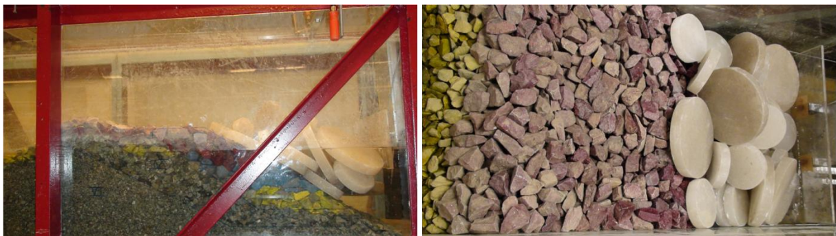
Figure 21 - Typical ice rubble formation in front of the breakwater during the tests with circular shaped ice. Test 57
