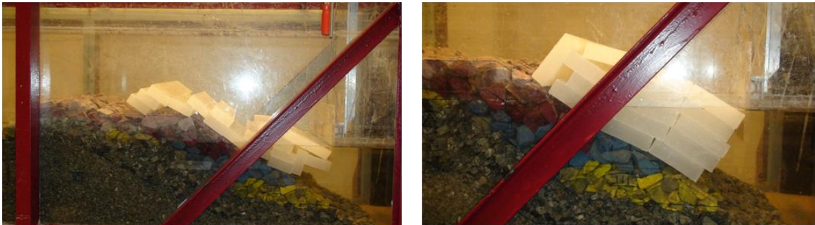
Figure 24-Accretion on the slope with (left) and without (right) previous ride up. Tests 24 (left) and 27 (right).
