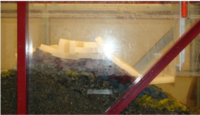
Figure 22-Test23: Typical ride up phenomenon
