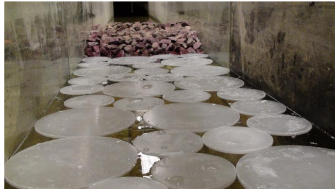
Figure 19 – Aspect of the circular shaped model ice the flume before test 49
