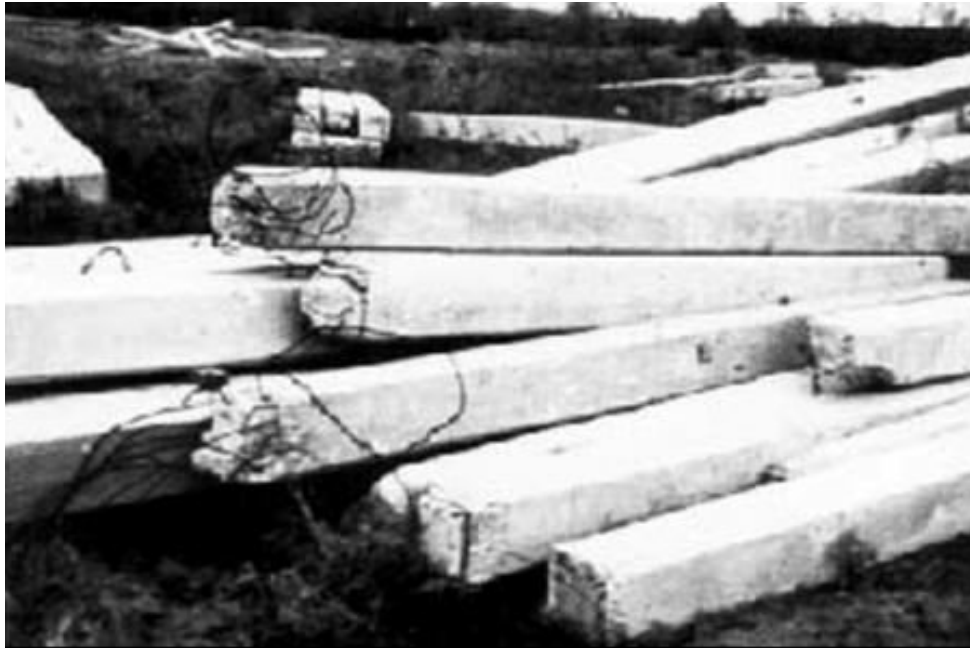
Figur 18 Skade betongpeler grunnet ramming under vanskelige grunnforhold (Foundation-Engineering 2011).
