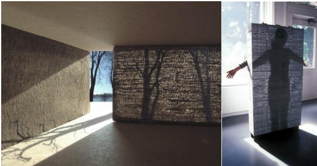
Figure 26. Translucent concrete used for architectural and daylight control functions (Perera 2012).
