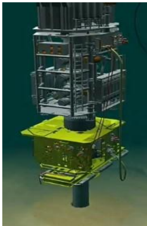
Figure 1-1 The BOP, wellhead and soil-conductor system
