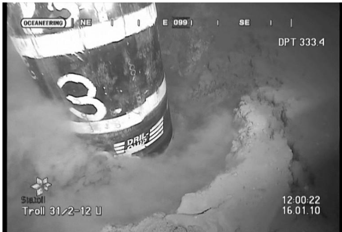
Figure 1-4: Troll well 31/2-12 U Drilling with BOP
