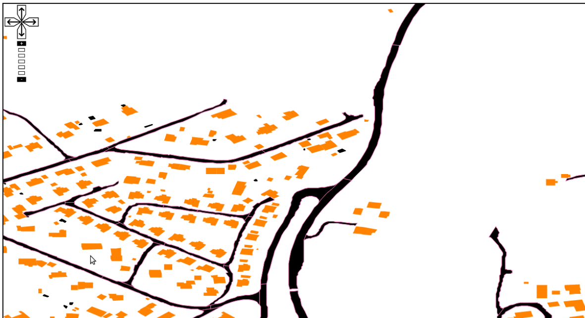
Figure 19: The styling is completely controlled by the client, which means that a change in the CSS, e.g. road colour fill to black, will be reflected in the map client (d), with no modification on the server.
