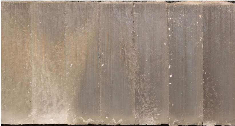
(a) Ice 2, series 5000. Ice-sheet thickness = 140 mm. This cross section has been sawn into 40 mm wide pieces in the vertical direction.
