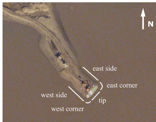
Figure 1: Orthophotography of Barryneset with the nomenclature of the different zones of the breakwater – Summer 2006
