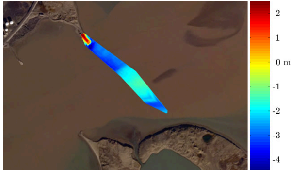
Figure 3.10: Seabed elevation map of Sveasundet – 25 July 2006 – Courtesy of Norges Geologiske Undersøkelser (NGU)
