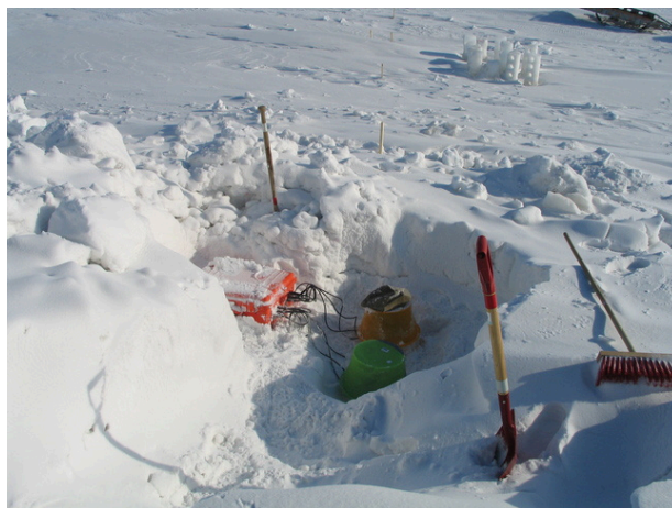
Figure 4.12: Set-up of the stress sensors. Datalogger in orange box – 26 April 2007 (week 17)
