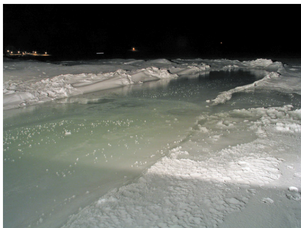
Figure B.54: Surface water on top of the hinge zone after holes were drilled, breakwater tip, looking toward the east corner, sea height = 0.5 m – 23 January 2007 (week 4)
