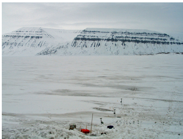
Figure B.77: The snow layer was rotting and the first meltwater ponds are starting to form. In the foreground the stress sensors with battery and logger. The three poles on the ice are DGPS rovers. The picture was taken from the cabin in the direction of Ispallen – 17 May 2007 (week 20)
