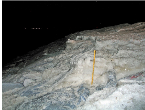
Figure B.24: Along the breakwater tip the ice foot was 40 cm high, looking toward Kapp Amsterdam, sea height = -0.6 m – 23 November 2006 (week 47)
