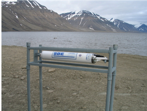
Figure 4.6: Tide gauge mounted on the steel frame
