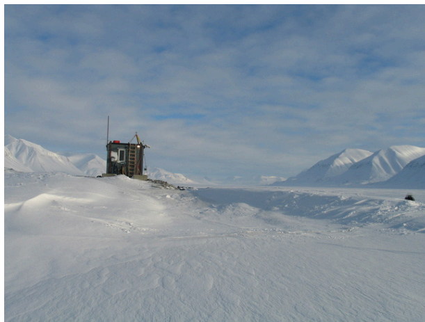
Figure B.68: Two snowdrifts had formed on the lee side of the cabin during the winter – 27 March 2007 (week 13)
