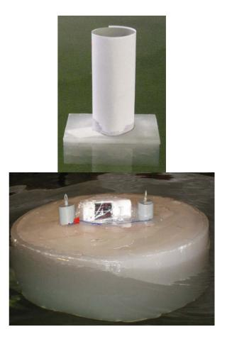
Figure 3. Test set up and illustration of position measurements. Photos of iceberg models.
