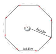
Figure 1. Configuration of eight sonars around an installation. R is the preferred distance from installation to the fence while L is the required footprint length for one sonar. Red dots indicate where the sonars should be located.
