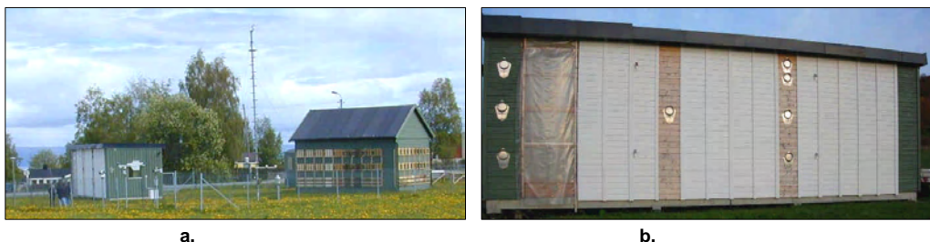
Figure 1. a) The Voll test field of NBI and NTNU with the two test houses and the meteorological mast. b) West facing façade. Wetness and temperature sensors are located close to the WDR gauges in the painted areas.
