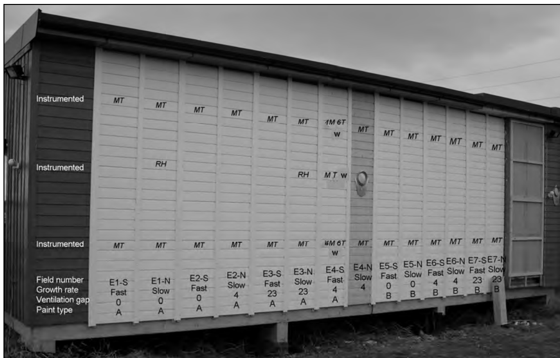
Figure 3.8. East facing wall of the test house. Letter codes correspond to Figure 3.7.
