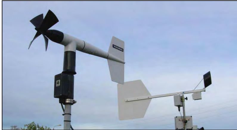
Figure 3.4. Wind measurements, the propeller measures wind velocity (m/s) and the two vanes measure wind direction (in degrees). The rotating WDR gauge at the back measures WDR in the main wind direction.
