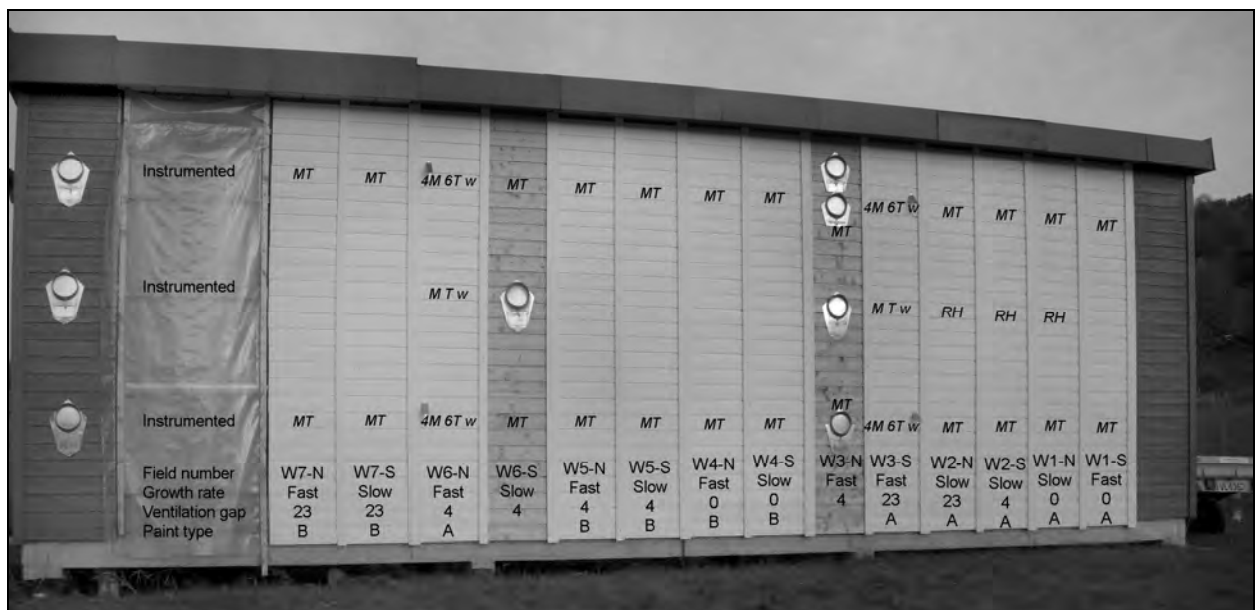
Figure 3.7. West-facing wall of the test house. Letter codes indicate design, material qualities and instrumentation of the different sections. 8 WDR gauges are mounted on this façade.
