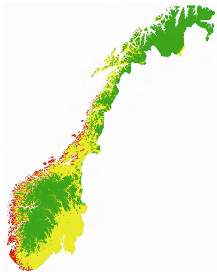
Figure 2.2. Risk for rot map for Norway based on Scheffer's index (Lisø et al. 2006).
