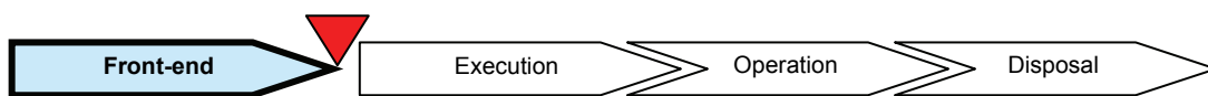
Figure 2.1 On the timeline, the dissertation is limited to covering the front-end (idea-, pre-study, and pre-project phase, often referred to as the early phases) up to the point where the decision makers (the owners) perform the final approval of a project (the GO/NO GO decision).
