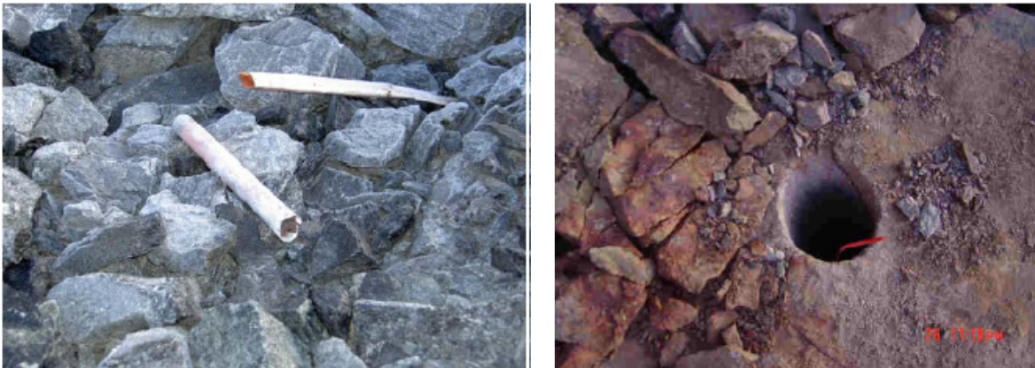
Figure 7 Left: Misfires in the muckpile. Right: Bottom of hole made visible during bench cleaning. Remaining Nonel shock tube indicating possible misfire. Photos: BEF [33].
