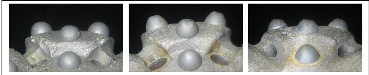
Figure 42 Different wear flats after 60 drms at Site 1. From left; Spherical, Semi ballistic and Ballistic.
