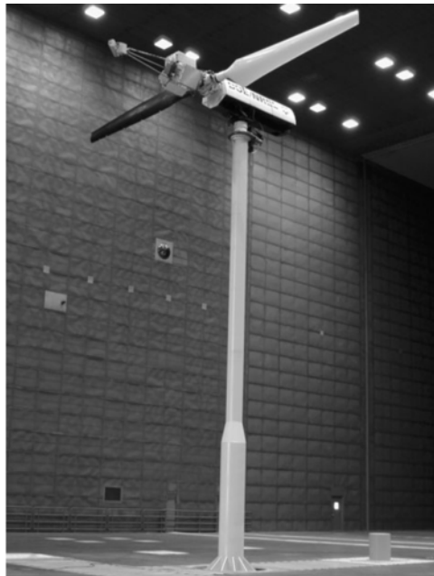
Figure 2. NREL wind turbine in the NASA Ames wind tunnel. (From Schreck, 2001) 13
