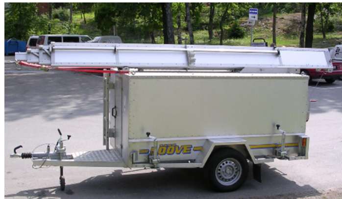
Fig. 27. Roadside traffic data collection.
