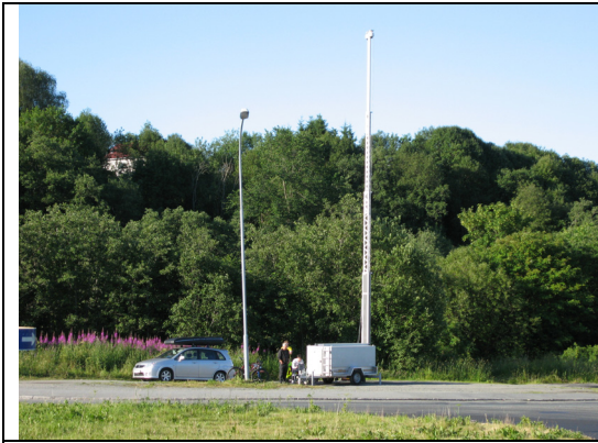
Fig. 28. Trailer with 15 meter pole for roadside video recordings.
