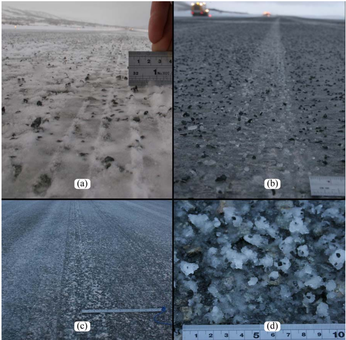
Figure 3-11. Tire tracks on the decaying contamination layer. (a) During the friction measurements at 11:42. The sand particles remained embedded in the track. (b) Friction measurement at 13:13. At this time, most particles broke loose together with ice fragments. (c) Fragmentation of the contamination layer by a landing Dash-8 at 13:21. (d) Detail of the fragmentation. Asphalt aggregates have become visible. Note that most fragmented pieces contain one or a few sand particles.
