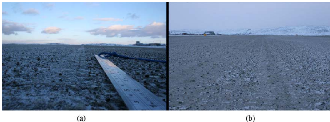
Figure 9-6. Tracks on newly applied freeze bonded sand. (a) The track from a BV-11 test tire. (b) The track of a Beach King Air 200. Both tracks show that large particles broke loose under the action of the tire.
