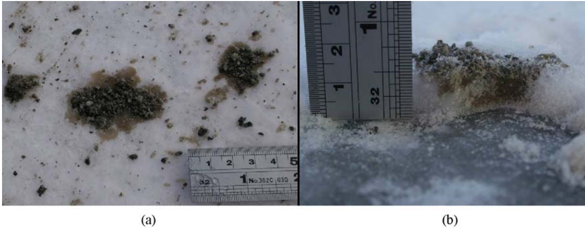
Figure 9-4. A top view (a) and side view (b) of warm pre-wetted sand that is applied on compacted snow.
