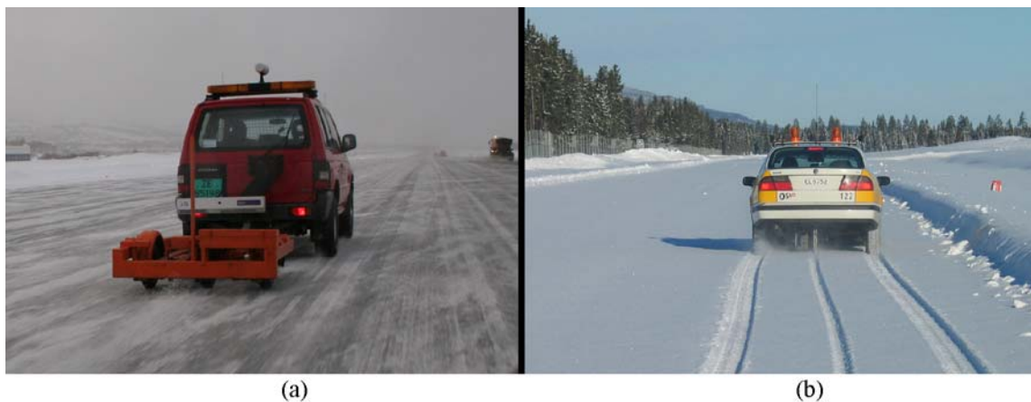
Figure 2-1. Two friction measurement devices used in Norway: (a) the Skiddometer BV-11 and (b) the Saab Friction Tester.
