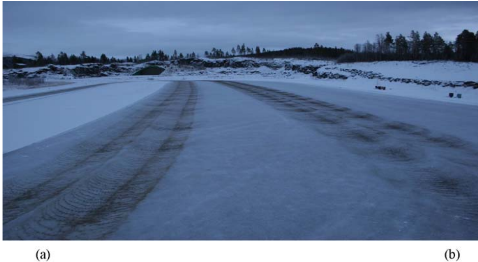
Figure 9-7. Overview of the test beds: (a) freeze bonded sand and (b) loose sand.
