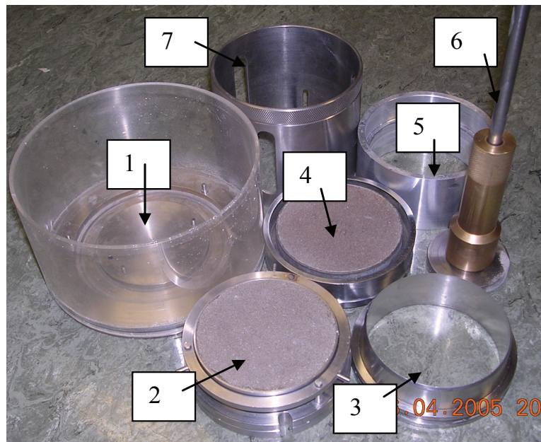
Fig. B.2 Accessories for specimen build-in for compression test
