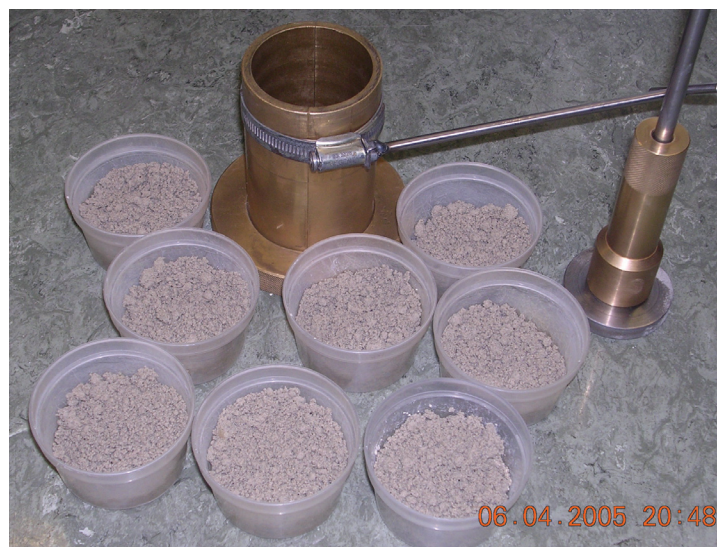
Fig. B.1 Accessories for specimen build-in in laboratory
