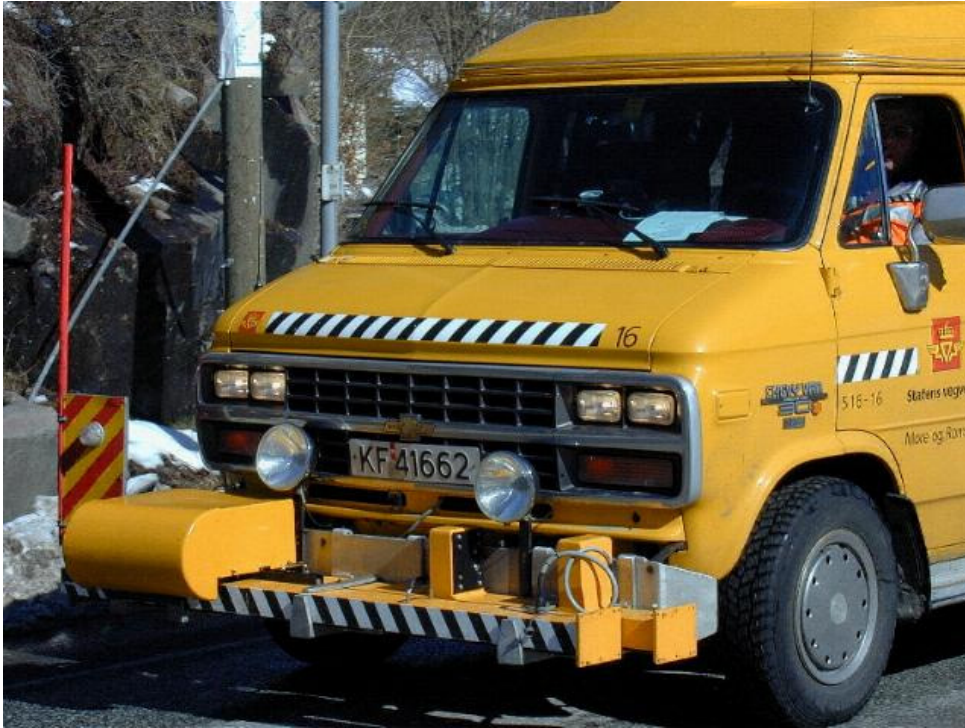
Figure 4-14 Photo of van with ALFRED laser/ultrasound device for roughness and rut depth loggings 104
