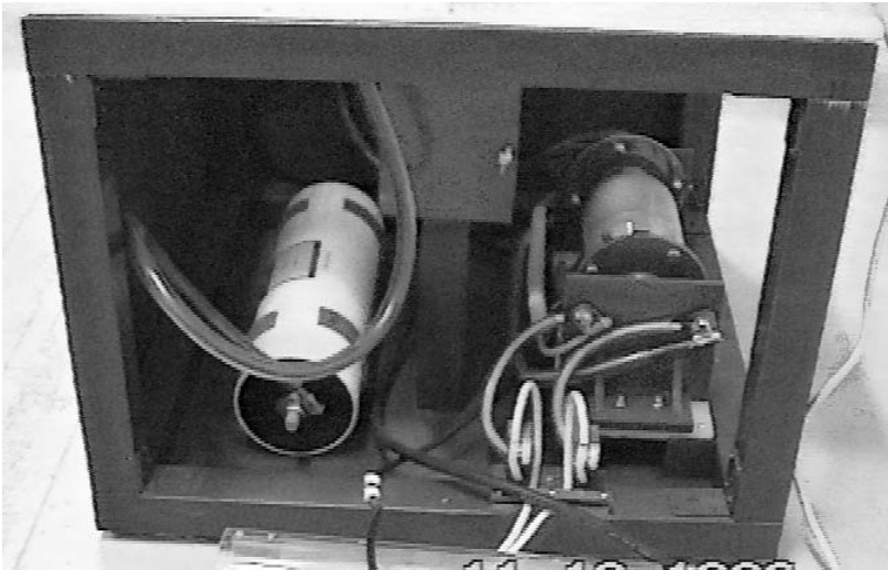
Figure 6-15: Tesla coil components
