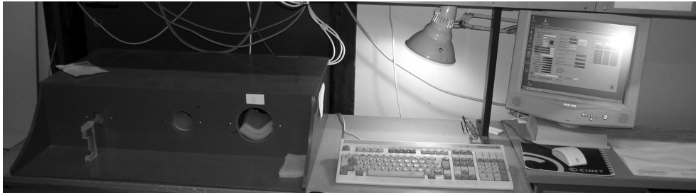
Figure 67 Pick-up coils for susceptibility measurements (to the left) in the NGU laboratory.
