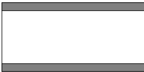
Figure 2.3 : HAZ along long edges
