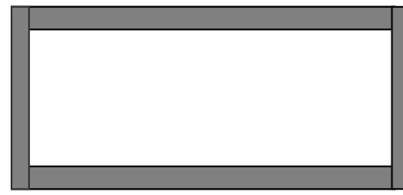
Figure 2.2 : Heat affected zones of a plate that have been conventionally welded, (HAZ along all edges)
