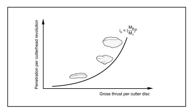
Figure 3.1 General progress of a penetration test curve.
