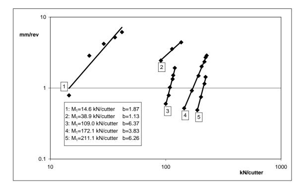
Figure 3.2 Plot of some penetration tests.
