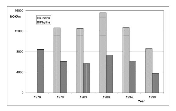
**Figure 3.4** *Predicted excavation costs for a 3.5 m diameter TBM with 394 mm cutters. Price level of January 1999 [18].*
