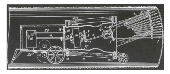
Figure 2.1 The patented tunnel boring device by Mr. I. Bøhn.
