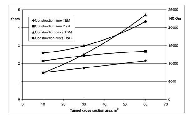
**Figure 2.3** Total construction time and total construction costs (1999 price level) for TBM and drill and blast tunnelling. Tunnel length 6 km. Rock conditions as in Figure 2.2 [18].
