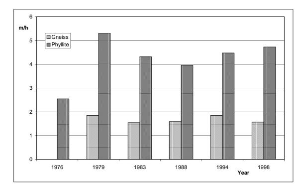
**Figure 3.3** *Predicted net penetration rate for a 3.5 m diameter TBM with 394 mm cutters* [18].
