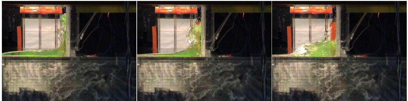
Figure 8.29 Water overturning and breaking after the impact. Nominal incoming waves with \lambda/D = 10.1 and H/D = 0.808 .
