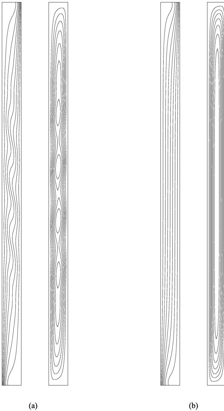
Figure 3.5. Possible flow patterns in a glazing cavity where the height to width aspect ratio is 20: (a) Ra = 10^4 ; (b) Ra = 5 \times 10^3 . In each figure the left-hand diagram displays temperature contours, and the right-hand diagram displays streamlines.
