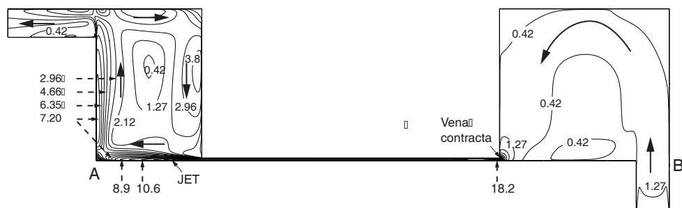
Figure E.3: Velocity contours at 0 rpm, axial Reynolds number of 12000 and clearance 0.552.
