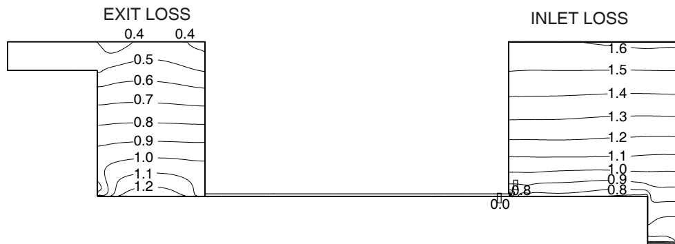
Figure E.9: Entrance and exit loss based on static pressure. 2250 rpm, Re_z = 4000 , S1/R2 .
