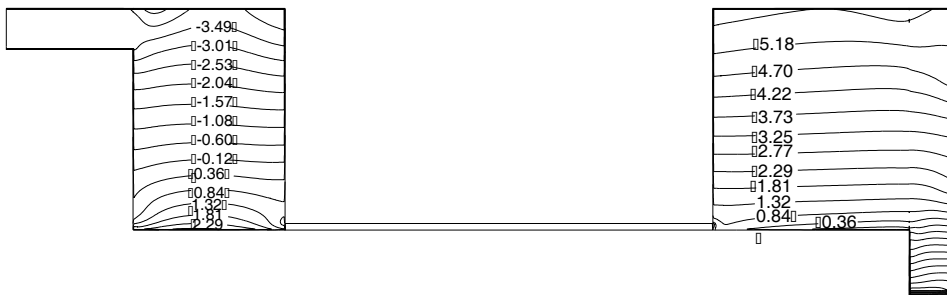
Figure E.11: Entrance and exit loss based on static pressure. 10000 rpm, Re_z = 5000 , S1/R2.
