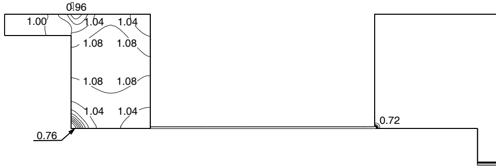
Figure E.7: Entrance and exit loss based on static pressure. 0 rpm, Re_z = 12000 , S1/R4.
