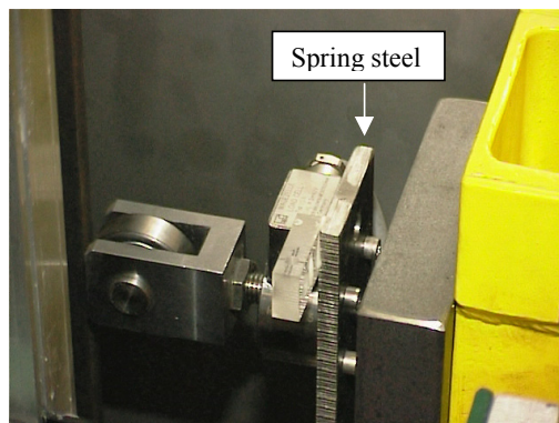
Figure 4.8: The load cell installed on the spring steel
