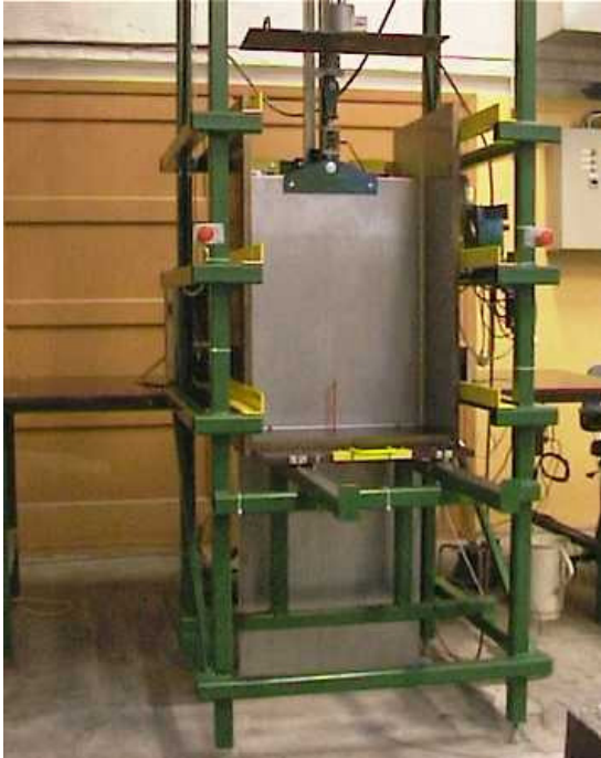
Figure 4.3: The vertical slipform rig.
