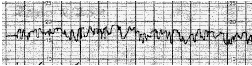
Figure 5.2: Surface profile for a new panel. The distance between the horizontal grid lines is 1\mu\text{m} and it is 250\mu\text{m} between the vertical grid lines. R_a = 0.9\mu\text{m} .
