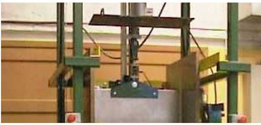
Figure 4.6: The lid for pressurizing the concrete.
