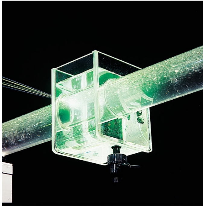
Figure 4.23b LDA measurements in oil-water flow in the Model Oil Facility.
