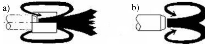
Figure 2-9 Internal recirculation: (a) recirculation cup, (b) jet-flow induced (Røkke, 1994)
