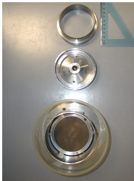
Figure 3–3: Photos of the incremental loading oedometer apparatus together with metal rings used at NTNU by the author.
