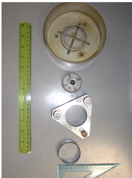
Figure 3–3: Photos of the incremental loading oedometer apparatus together with metal rings used at NTNU by the author.
