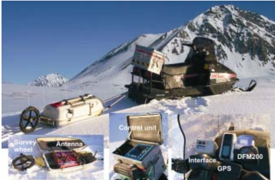
Figure 4-4 Setup of the Snowradar, GPS and DFM 200 receiver.
