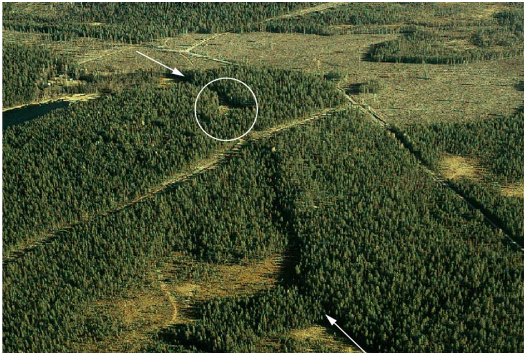
Fig. 5.7 Late- or postglacially developed fault scarp at Röjnoret, some 40 km to the west of Skellefteå, Sweden. The scarp runs diagonally across the photograph, from upper left to lower right, as indicated. The trench shown in Fig. 5.8 is encircled. Photo: Robert Lagerbäck. Reproduced from Bargel et al. (1999b).
