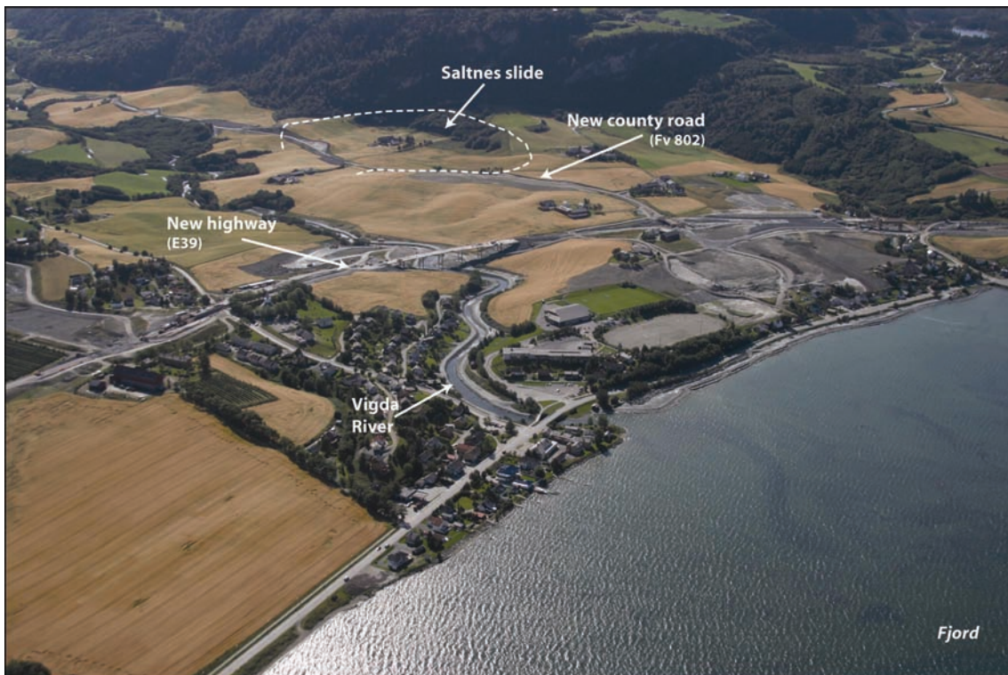
Fig. 2. Buvika during construction of highway E39. The photo is taken towards southwest (Photo: the Norwegian Water Resources and Energy Directorate, NVE).
