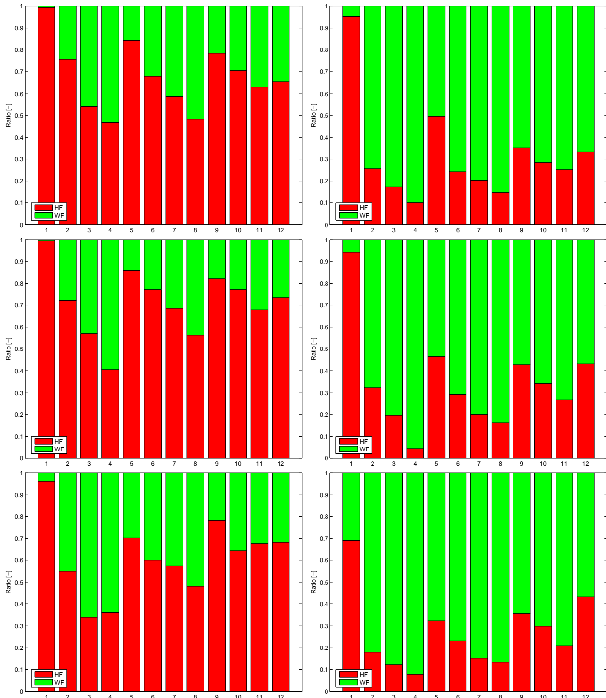
Figure 5.23: Ratio of WF (top) and HF (bottom) damage to total fatigue damage for midship section at full speed. Left= Ballast, right= Cargo. Row 1= Bow 1, row 2= Bow 2, row 3= Bow 3.
