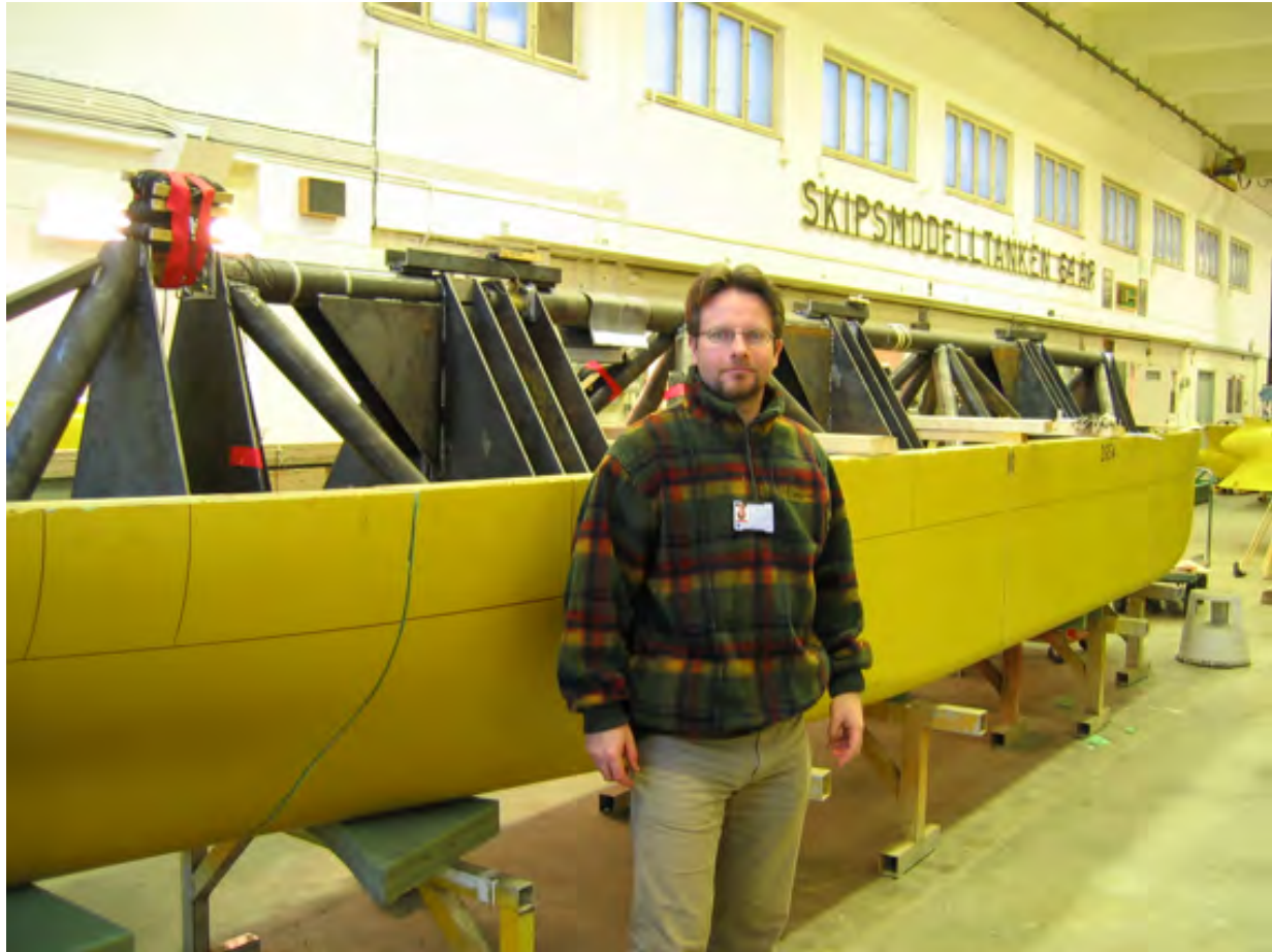
Figure 4.1: Picture of the 8.7m model with the steel frame and transverse triangular end plates, which defined the location of the flexible joints and global load sensors.
