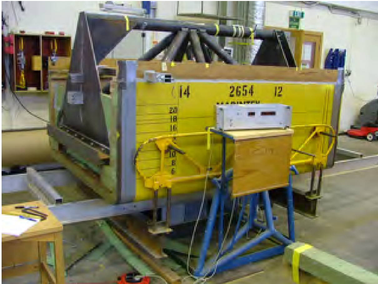
Figure B.2: Cradle with segment 4 and with the crystal clock shown in front.
