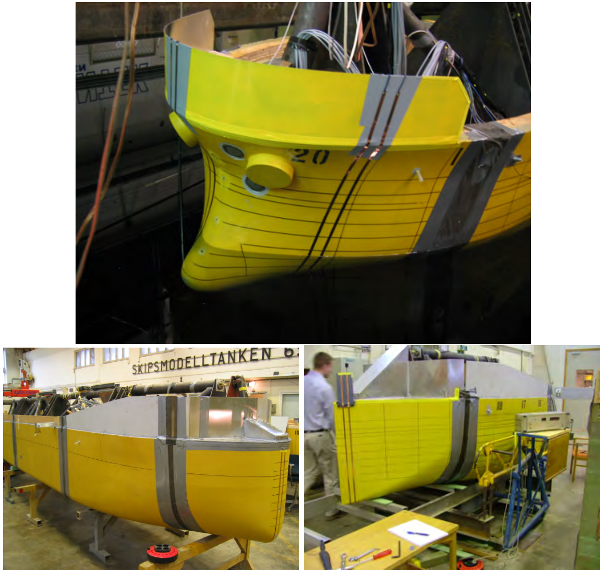
Figure 4.4: The three bows. Bow 1 = Upper, Bow 2 (cargo) = Lower left, Bow 3 = Lower right. Bow 3 (segment 5 and 6) is placed on the cradle. All bows have significant bilge radius (bottom flare).
