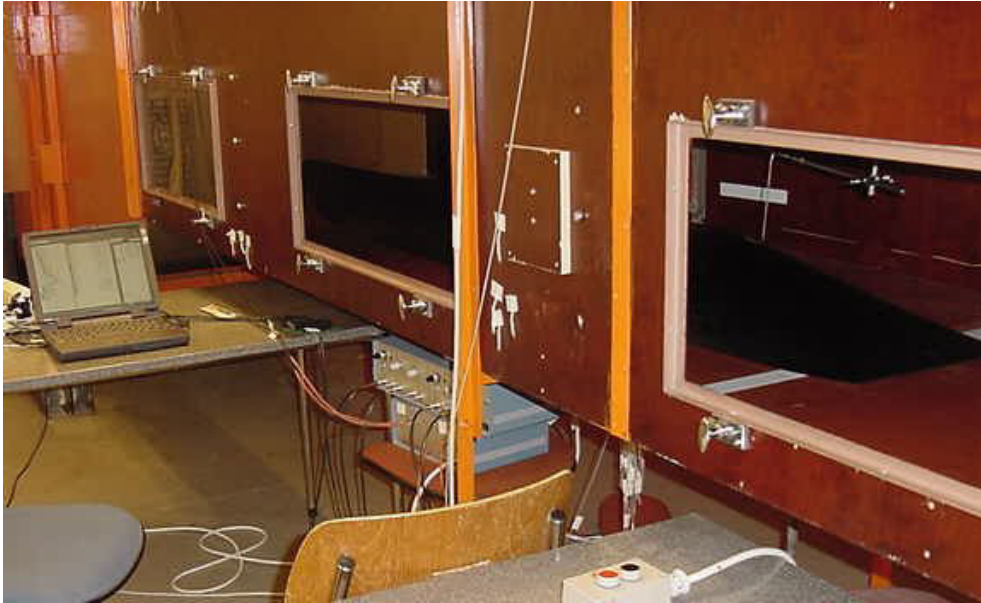
Figure 4.5: A picture of the wind tunnel with a ship model on the floor inside the tunnel. Pressure transducers, amplifier and data logging equipment is seen by the table.
