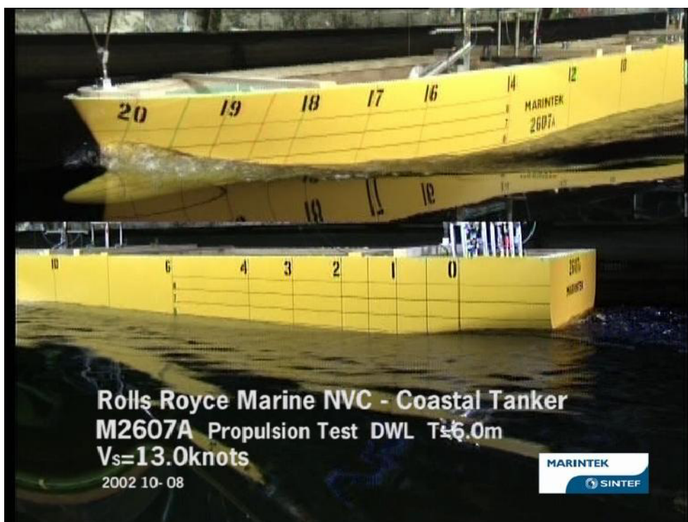
Figure 5.10: Picture of hull alt. 3 from towing test. Fn=0.24 .
