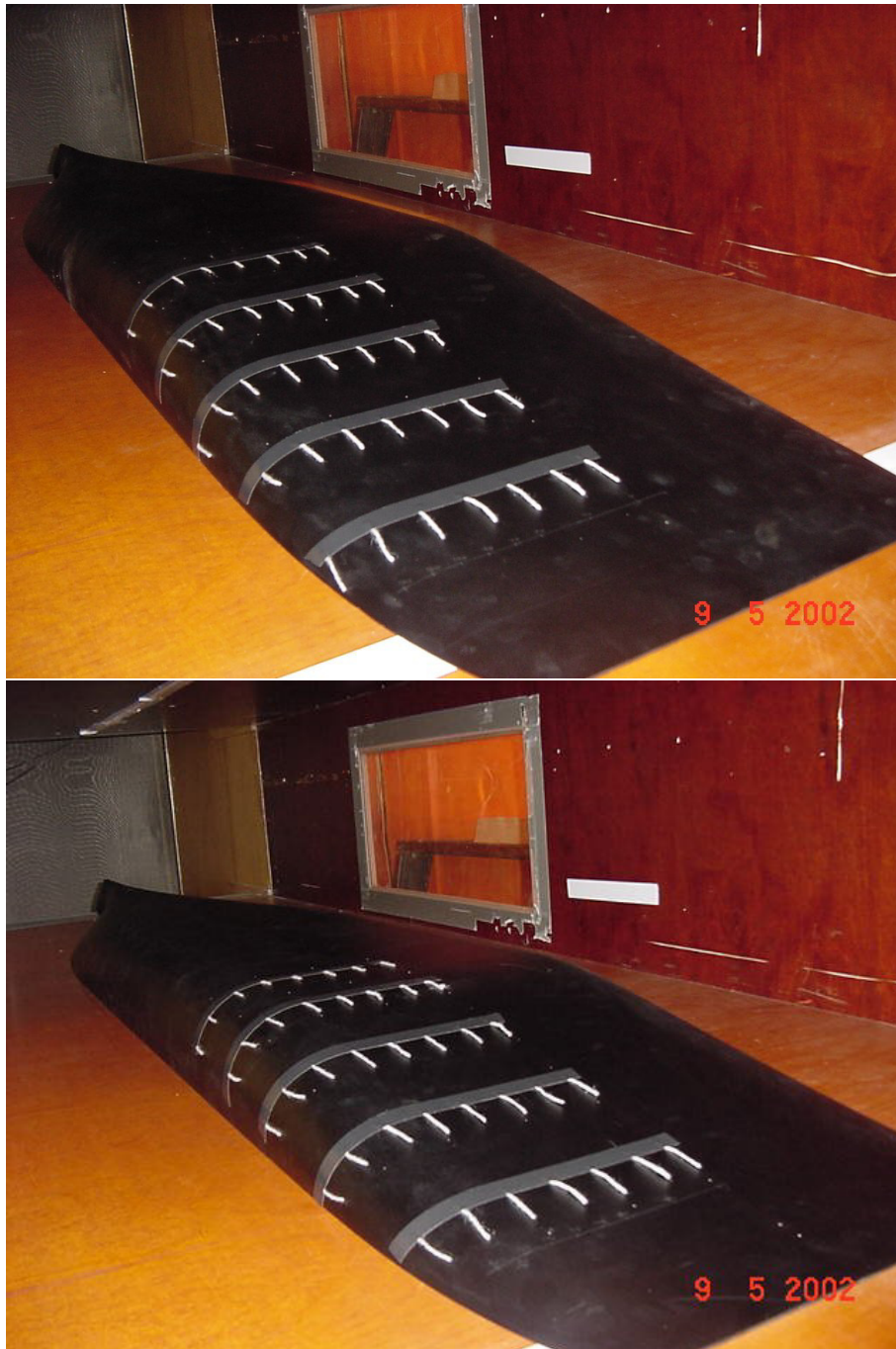
Figure 4.12: The picture on top shows tufts on the surface of Mod A. The bottom picture shows the same for Mod B. Both runs are done at 22 m/s.
