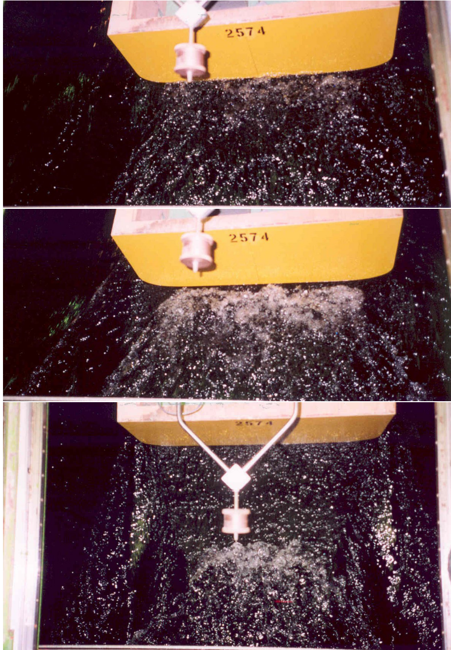
Figure 4.36: The figures show stern view of Mod B. Top: 19.1 kn ( F_n=0.28 ). Middle: 21.1 kn ( F_n=0.31 ). Bottom: 25.1 kn ( F_n=0.37 )
