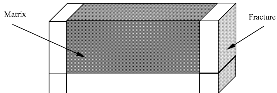
Figure 4. Equivalent dual-porosity model of 3x1x2 coarse-grid (model type-2 is converted).
