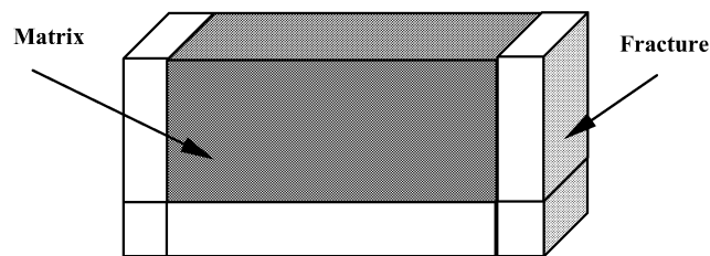
Fig. 7.4—Equivalent dual-porosity model of 3x1x2 coarse-grid. Fine-grid model is not shown. Also, fracture width is not shown to scale.
