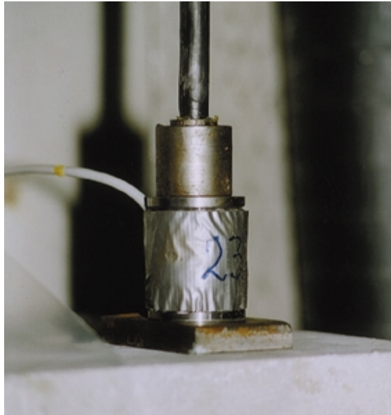
Load cell at the anchorage.
