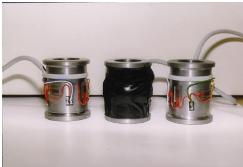
Strain gauges glued to load cells.
