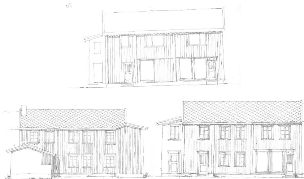
Figure 23-25: Sjøgata 41, survey of street façade 30.8.1977 (top); restoration plan for the backyard façade 29.3.78 (left) and street façade (right) by Bjørn Grimsby Arkitekt M.N.A.L in 1978. The restoration was based on a 1905 photograph and building parts in the façade which had not been altered during the 1960s modernization; (Vefsn municipal building archive)
