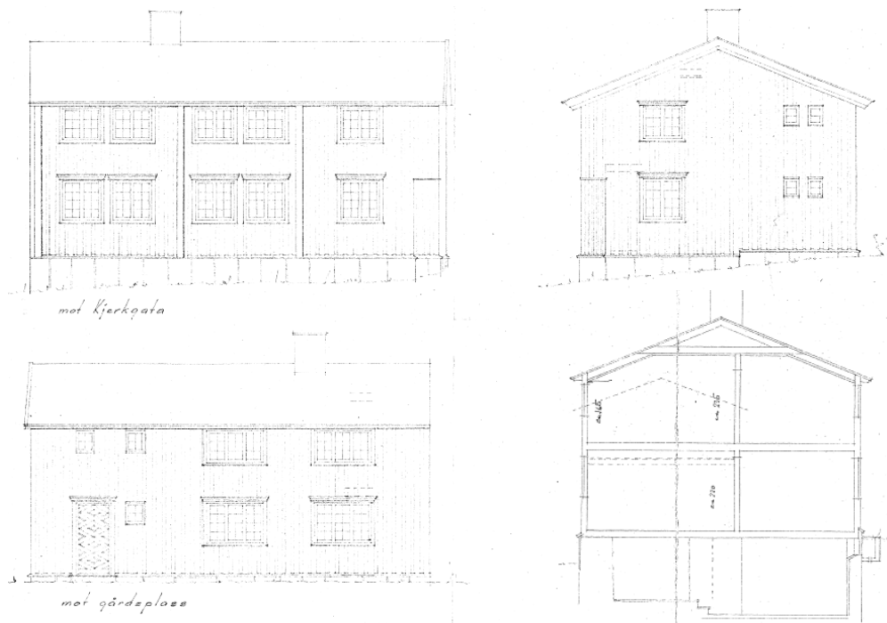
Figure 69-70: façade designs for Kjerkgata 60 (architect Stensaas referred to the plans as a “restoration” in his letter to Riksantikvaren ): street façade (upper left) northern gable wall (upper right) courtyard façade (bottom left). Figure 70, the section (bottom right, inserted) showing the new house, and the outline of the old dwelling marked with dots. Architect Johan Stensaas 7/2-54. (Røros municipal building archive)
