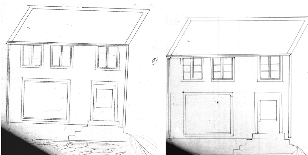
Figure 56-57: Kjerkgata 58, two alternatives for the upstairs windows in 1960. Riksantikvaren opted for the traditional design (right). (Røros municipal building archive)
