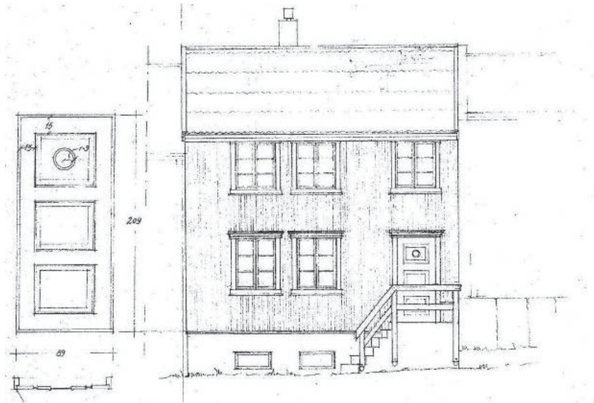
Figure 60: Design for the façade of Kjerkgata 58 by architect Seppo Heinonen, 1975, entrance door, original scale 1:20 (left) and street façade, original scale 1:50 (right). The design involved new windows and mouldings, a new entrance door and new steps and banister. (Riksantikvaren archive)
