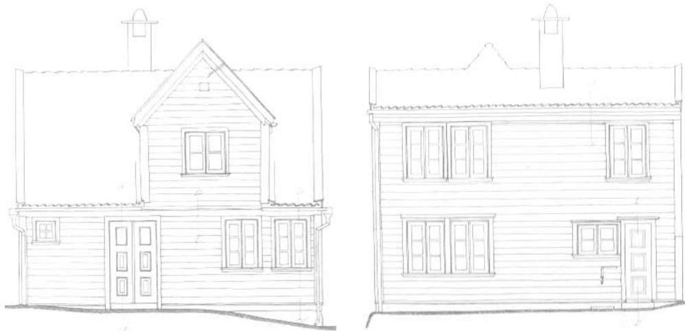
Figure 29-30: Fjæregrenden 16, north façade facing Fjæregrenden (left); south “garden façade” (right). Original scale 1:50, Gamle Bergen November 1943. (Gamle Bergen Museum archives)
