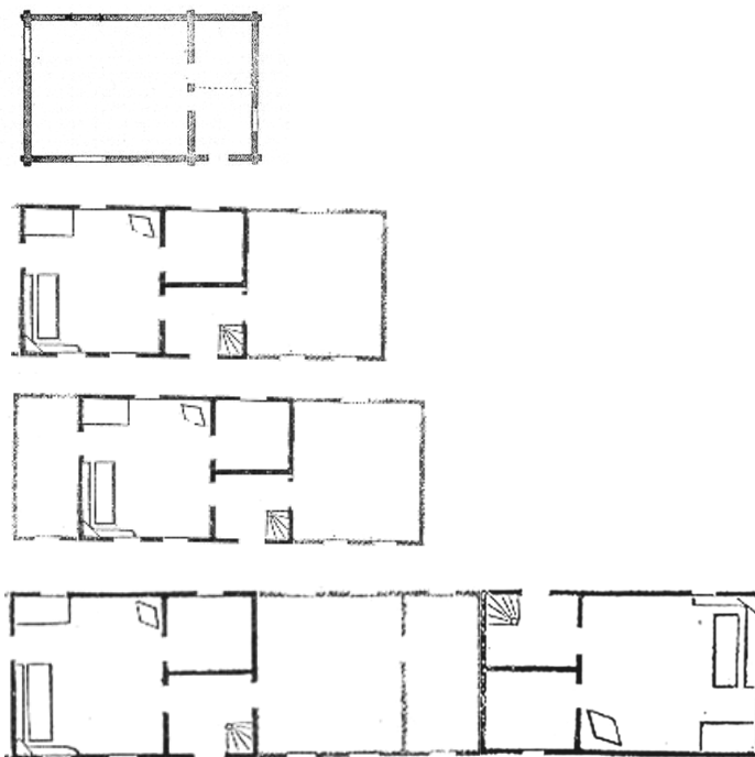
Figure 10: The development of the floor plan in Trøndelag vernacular according to Eilert Sundt. The three-room type, the paired room type with an added nystue ; the paired room type with an added “long chamber” ( langkammers ), and lastly the double unit, where the addition was in fact a separate unit (for the older generation) with a separate entrance and, in this case, no internal connection. (Eilert Sundt, Digitalarkivet)
