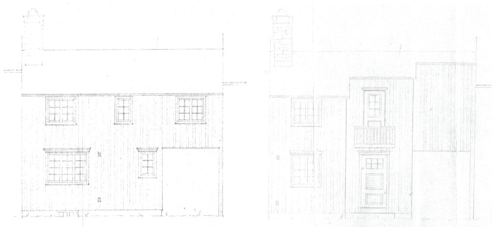
Figure 45-46: Kjerkgata 56, backyard façade, alternative plans for reconstruction. The altered proposition of 1952 was the basis for the reconstruction, although it became taller than Stensaas' plans proposed. Courtyard façade 25/2-1950 (left); courtyard façade 23/2-1952 (right); Architect Johan Stensaas. (Røros municipal building archive)
