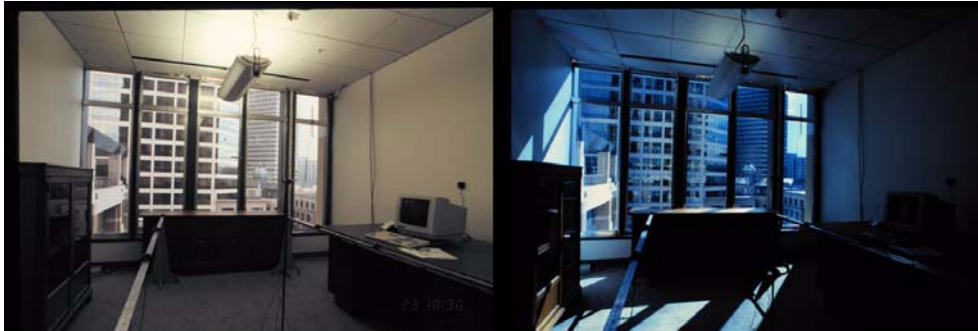
Figure 5-28: Electrochromic glazing tested at the Lawrence Berkeley National Laboratory, in transparent (left) and coloured (right) state.
