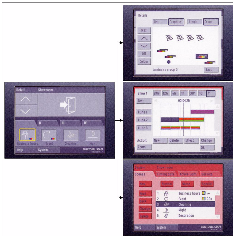
Figure 5-14: The Emotion touch panel; (left) main screen; (right) secondary screens for more detailed configuration.
